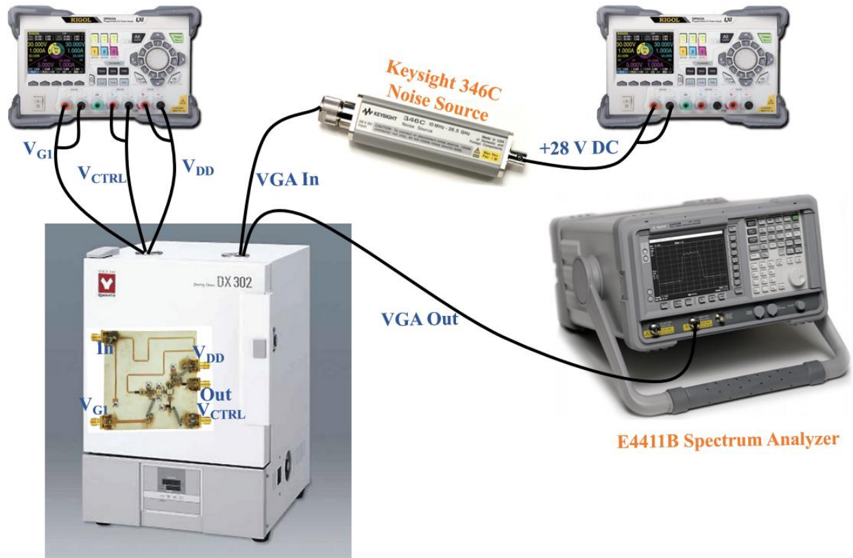
Fig. 4.2: Test setup for high temperature NF measurement [44]-[47], [49].
