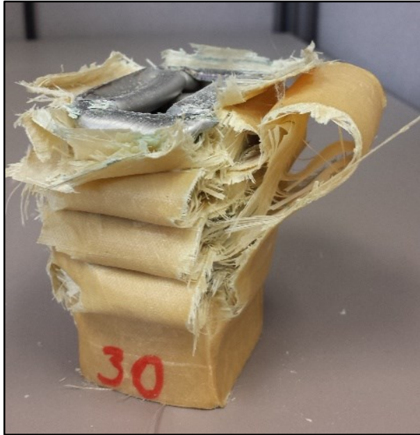
Fig. 2-6. One of samples with [90/\mp 30/0]_s stacking sequence which has delamination in one side
