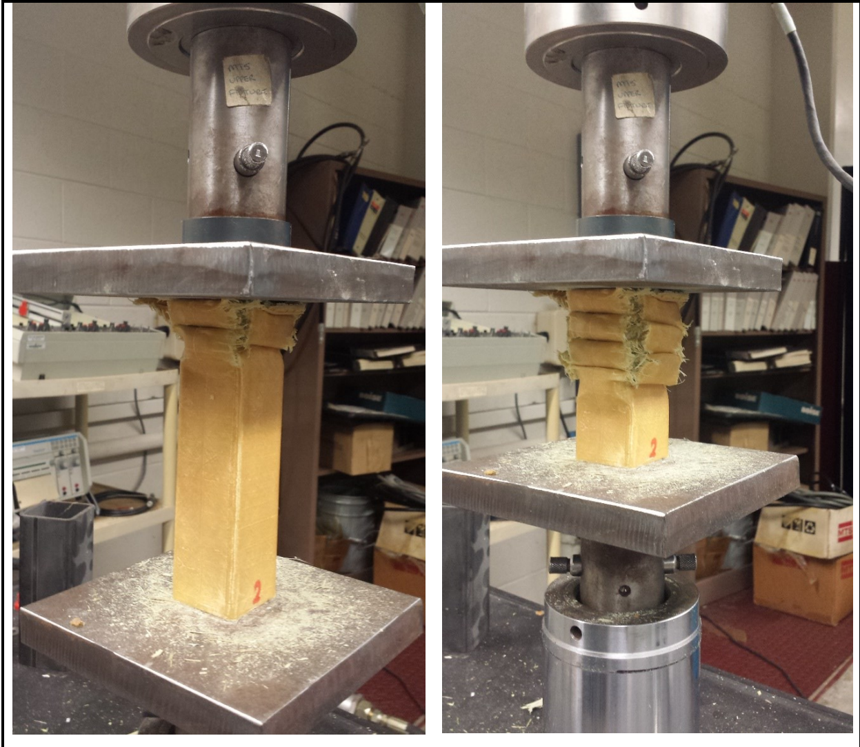
Fig. 2-2. Hybrid samples crushed up to 150 mm under quasi-static loading by hydraulic MTS 810 testing frame with 250 kN load cell
