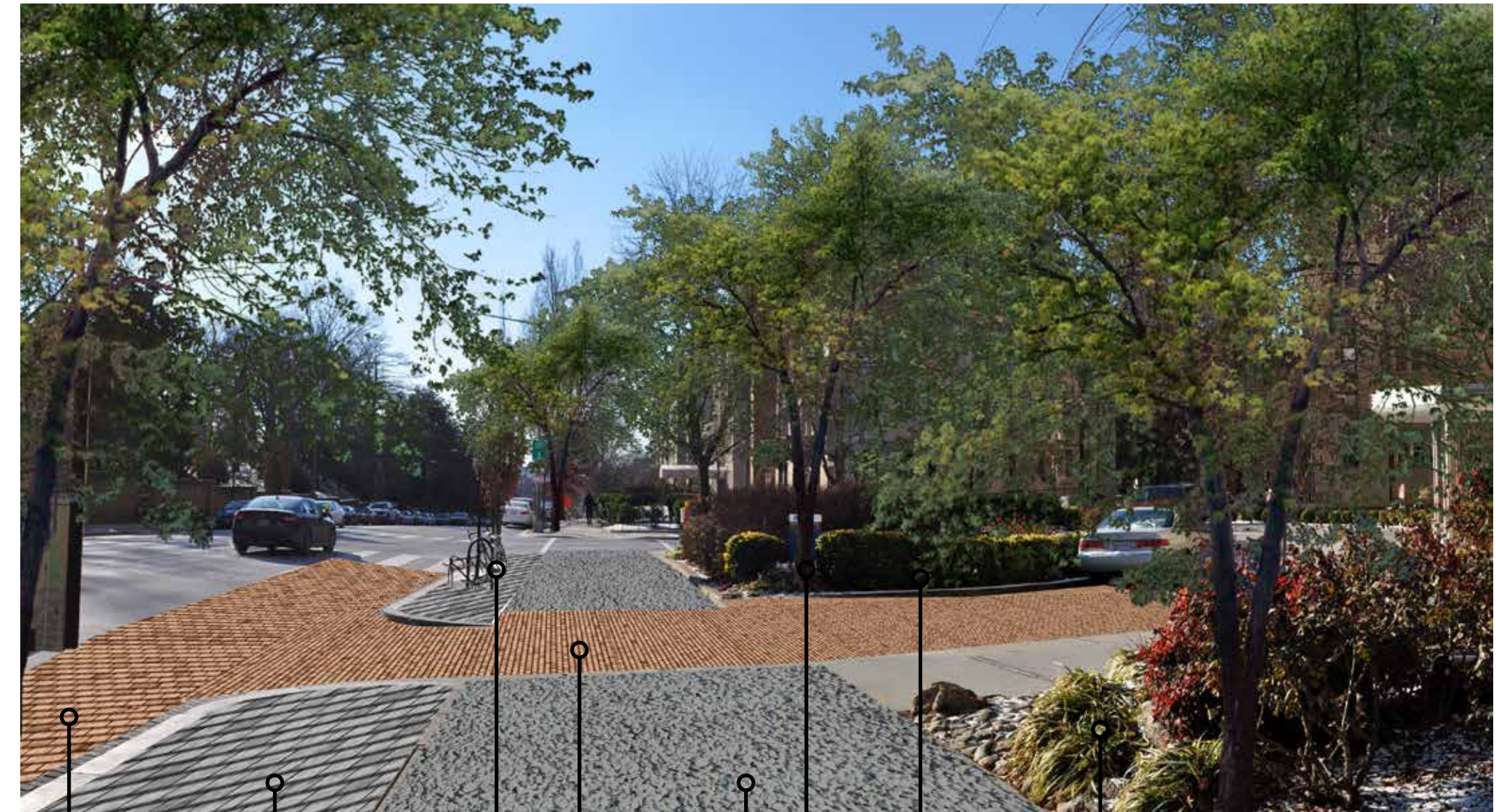
View A Sidewalk Perspective (See plan for reference) Permeable Pavement in Pedestrian Crossing Permeable Pavement in Vehicular Parking Areas Street tree Permeable Pavement in Driveway Street tree Bioretention in Open Area collecting water from driveway Bioswale
