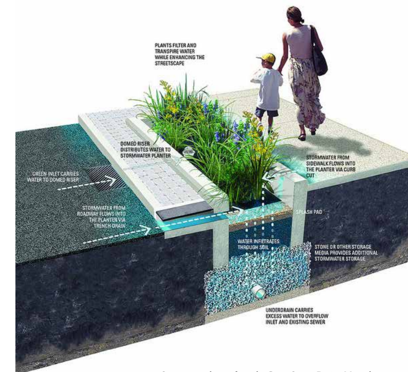
Stormwater planter, from the Green Streets Design Manual http://www.phillywatersheds.org/
