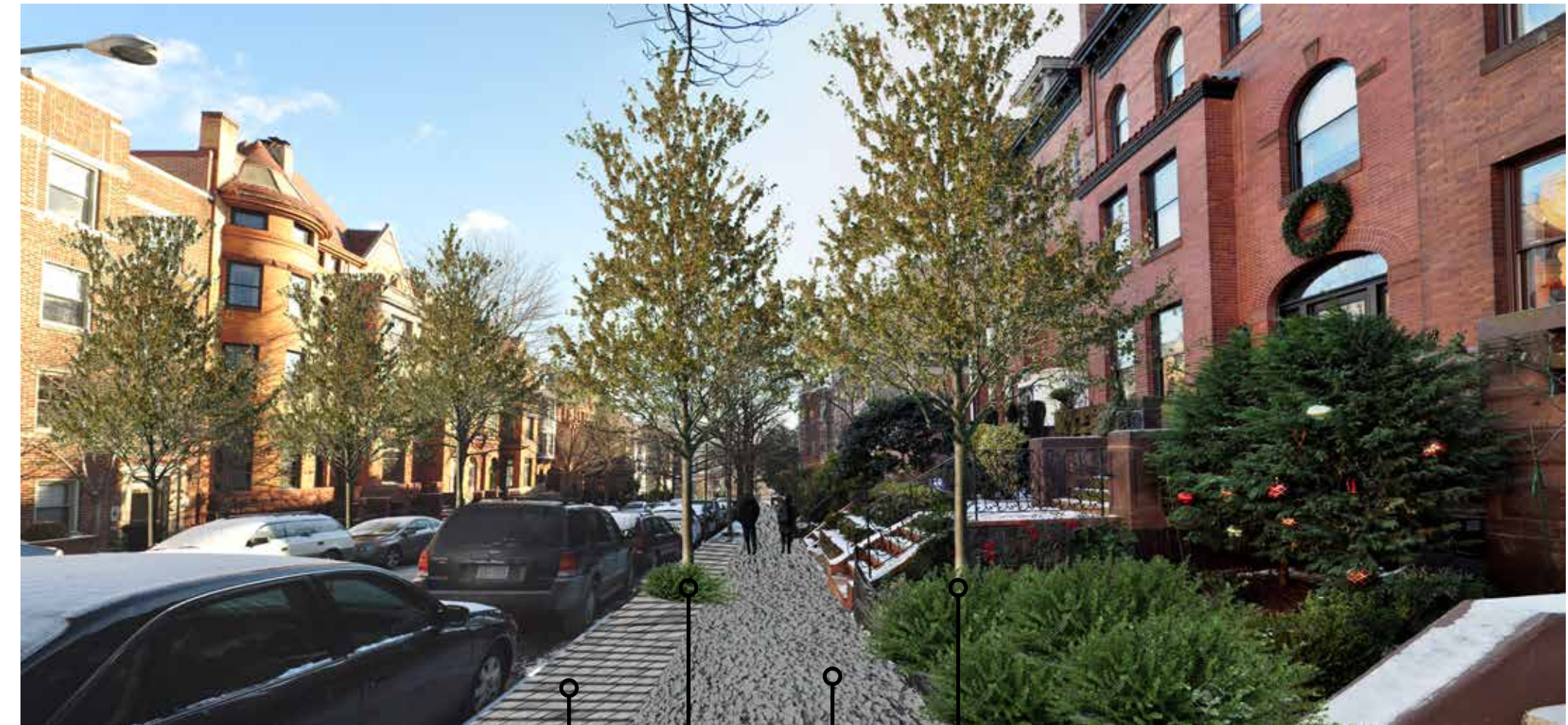
Permeable Pavement in Pedestrian Crossing Street tree Street tree Pervious Concrete View A Sidewalk Perspective (See plan for reference)
