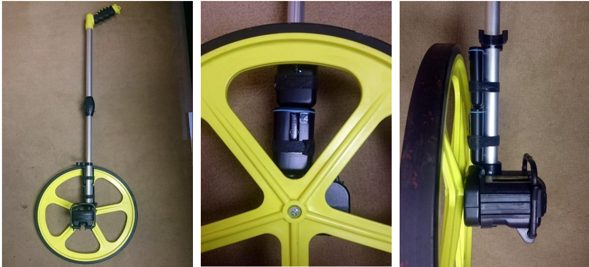
Figure 8. Arrangement of the GPS units attached to the trundle wheel.
