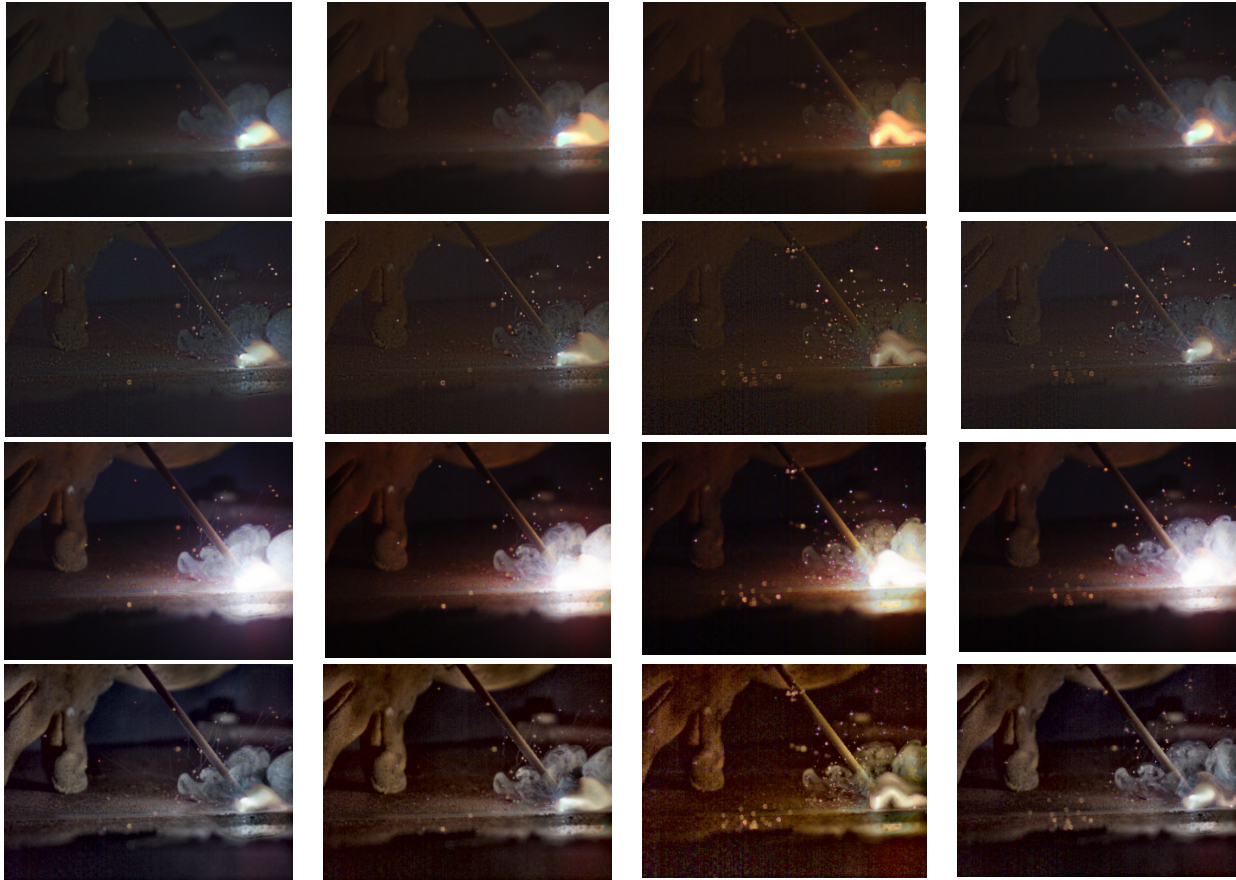
Figure 5-13. Arc weld video created with EMM method tone mapped via: Top Row. Griffiths Global. Top Middle. Griffiths Local. Bottom Middle. Reinhard. Bottom. Matlab's Histogram equalization method.
