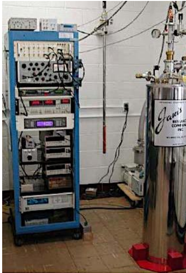
Figure 2.4 Picture of measuring setup. Equipment consist of a LakeShore 370 AC resistance bridge, Princeton Applied Research P124A analog lock-in amplifier, SR 830 digital lock-in amplifier, EG&G 7265 digital lock-in amplifier, Keithley 2400 source meter, Keithley 2000 multimeter, Yokogawa GS200 voltage sources, Cryomagnetics CS-4 superconducting magnet power supply. The steel can on the right is the cryostat system.
