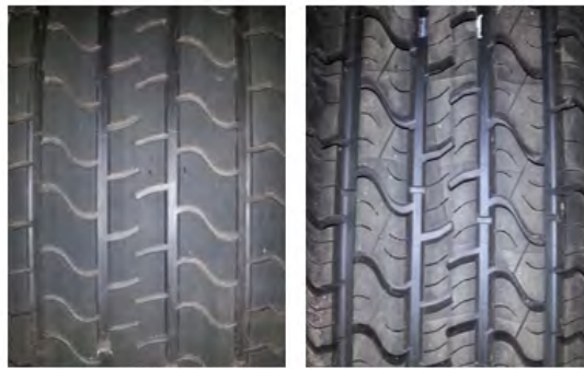
Figure 4.1: Tread pattern of the SRTTs. Left- Buffed SRTT with 1.6 mm tread depth. Right- Treaded SRTT with full tread depth of 7.97 mm.
