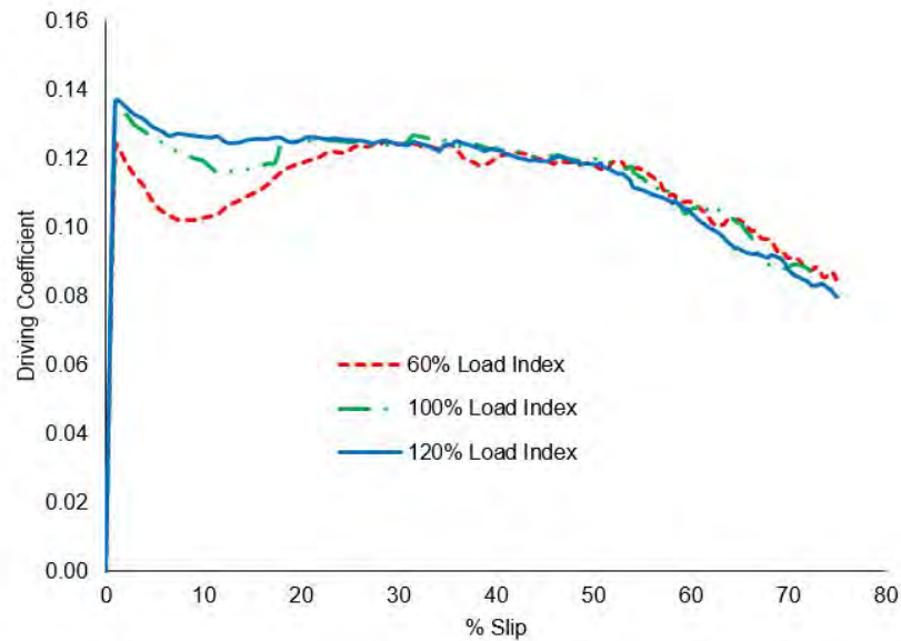
Figure 6.3: Effect of normal load on drawbar pull for the treaded SRTT on ice with 100% inflation pressure (242 kPa), from outdoor testing.
