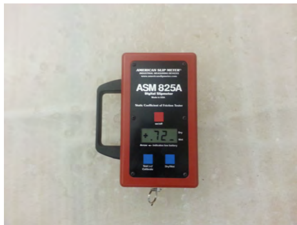
Figure 3.12: Slip meter employed to measure the static coefficient of friction of ice.
