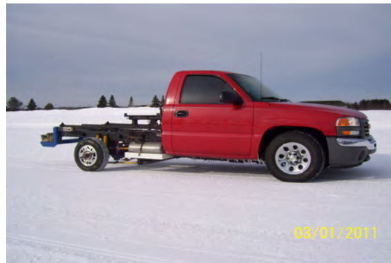
Figure 3.14: Mobility Research Inc.s' traction truck employed to evaluate tire performance on ice. Reprinted with permission from Mobility Research Inc.
