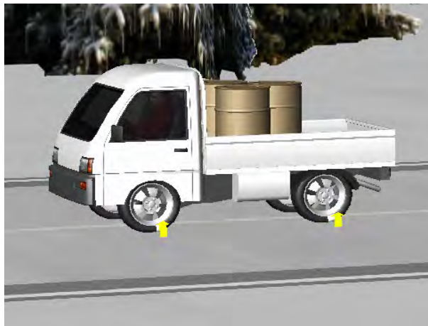
Figure 8.1: Compact utility truck model in TruckSIM® used for simulating tractive and braking performance on ice.
