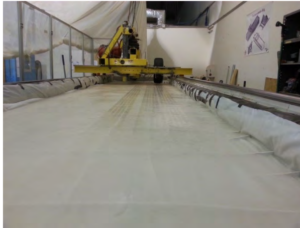
Figure 5.2: Smoothing and polishing of the ice surface by the tire footprint after testing on three parallel tracks.
