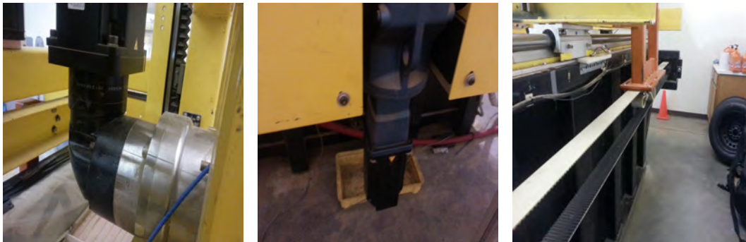
Figure 3.3: Drive train system of the Terramechnaics Rig. Left- Motor on the carriage to provide torque to the wheel; Middle- Motor used to control the longitudinal movement of the carriage; Right: Belt drive for longitudinal motion of the carriage.
