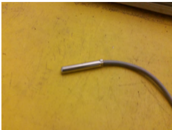
Temperature sensor of the ice making system.
