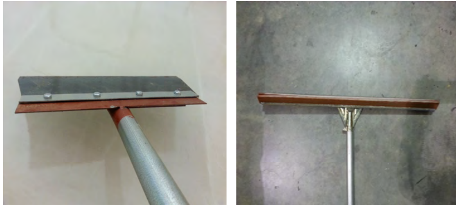
Figure 3.11: Tools used for resurfacing the ice surface in the test chamber of the Terramechanics Rig. L–floor scrapper and R–water squeegee.
