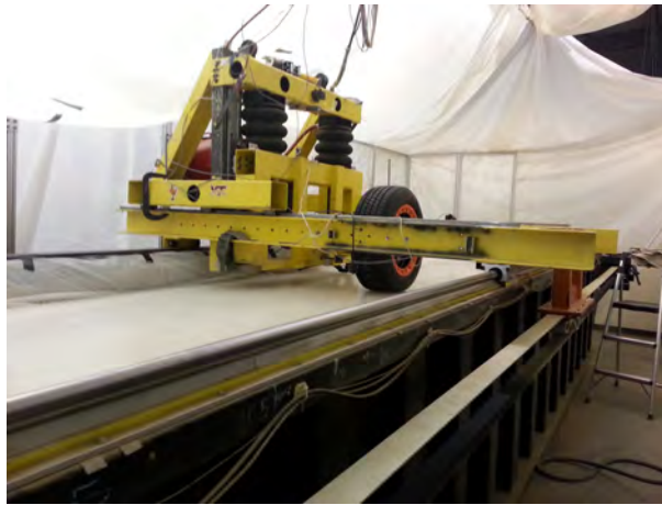
Figure 3.1: Terramechanics Rig at the Advanced Vehicle Dynamics Laboratory employed for evaluation of tire performance on ice.
