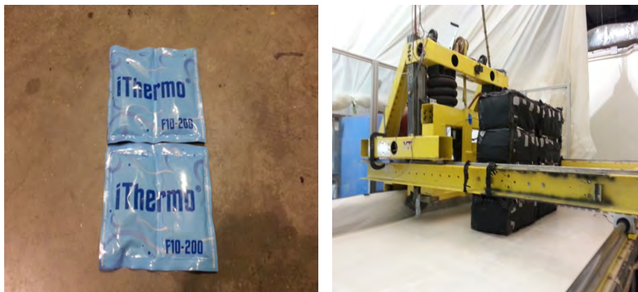
Figure 3.8: Left- ThermoCell from iThermo®. Right- Tire enclosure in operation on the Terramechanics Rig controlling temperature.
