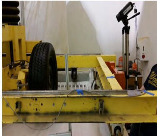
Figure 10.1: Infrared camera mounted onto the carriage of the Terramechanics Rig.
