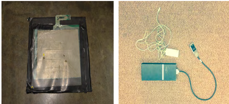
Figure 3.9: Left- Tekscan ® 3150 pressure pad. Right- Handle to connect the pressure pad to the computer.
