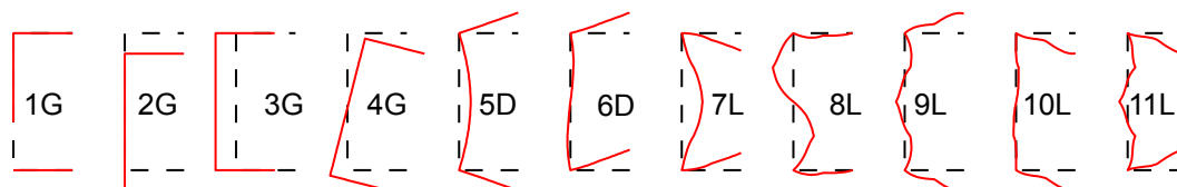
Figure 6.21: GBT mode shapes for Specimen 1, G global, D distortional, L local buckling
