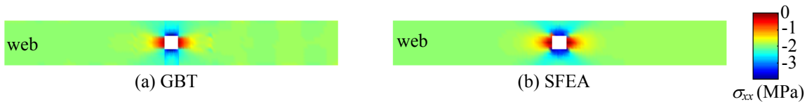
Figure 4.5: Local buckling example: first order analysis normal stress distributions: (a) GBT, (b) SFEA
