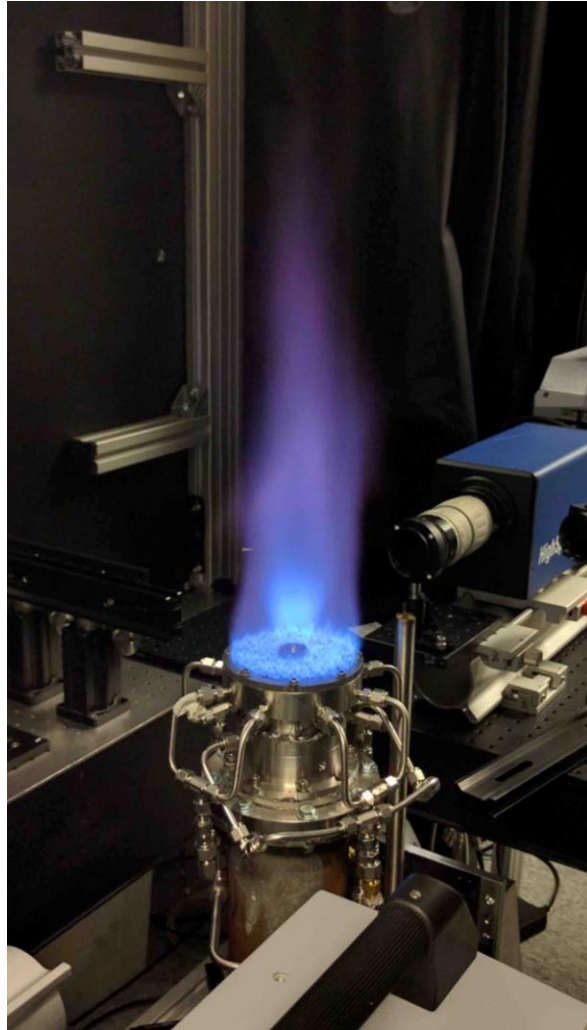
Figure 2.2. Photograph of HiPilot flame.
