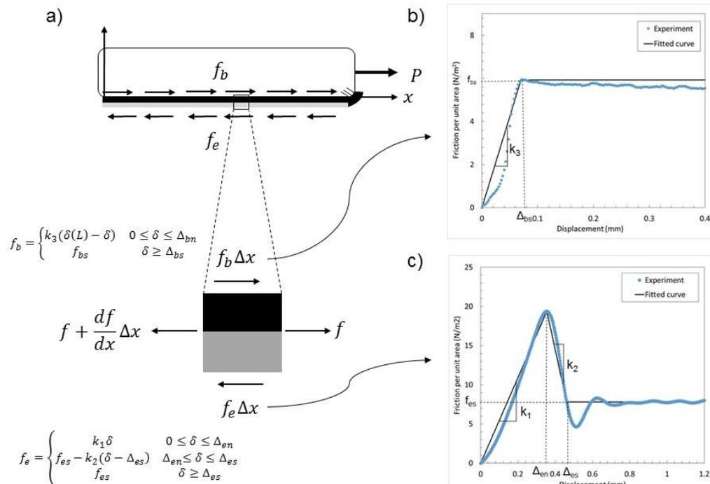
Figure 2. a) A differential element of an elastomer-coated fabric in contact with a substrate b) friction force between sled and backing fabric c) intrinsic friction response of elastomer with rigid backing
