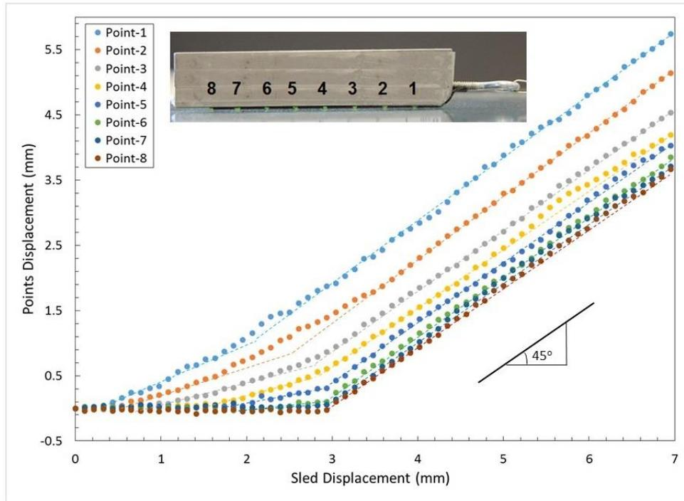
Figure 3. Displacement of different points and development of slippage zone across the length of strip. The least-square fits (dash lines) confirm the formation of transition and slip zones
