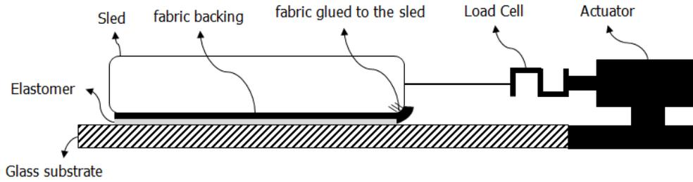
Figure 1. Schematic of experimental setup
