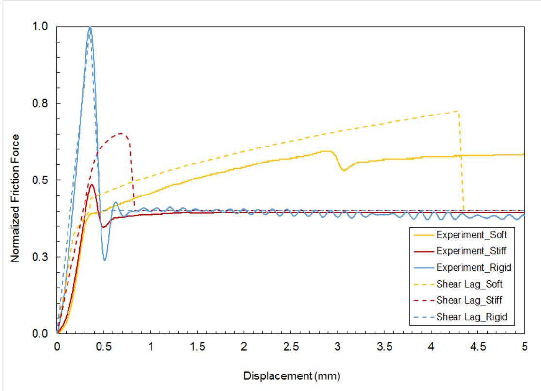
Figure 4. Force versus displacement curve of strips with three different backing stiffness
