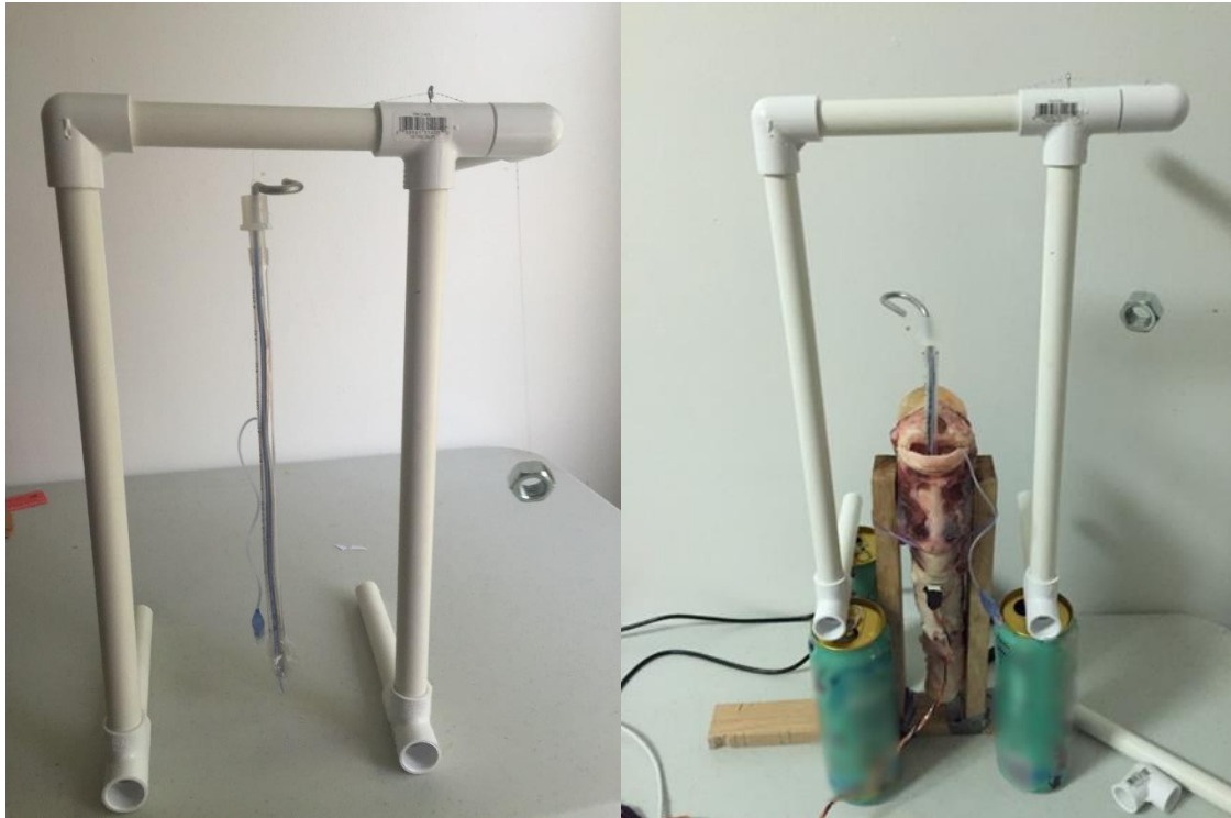
Figure 28. The gantry system for supporting and advancing the ET tube through the pig trachea. The ET tube is suspended by monofilament line attached to a counter weight. Marks on the monofilament line are used to assess insertion depth.
