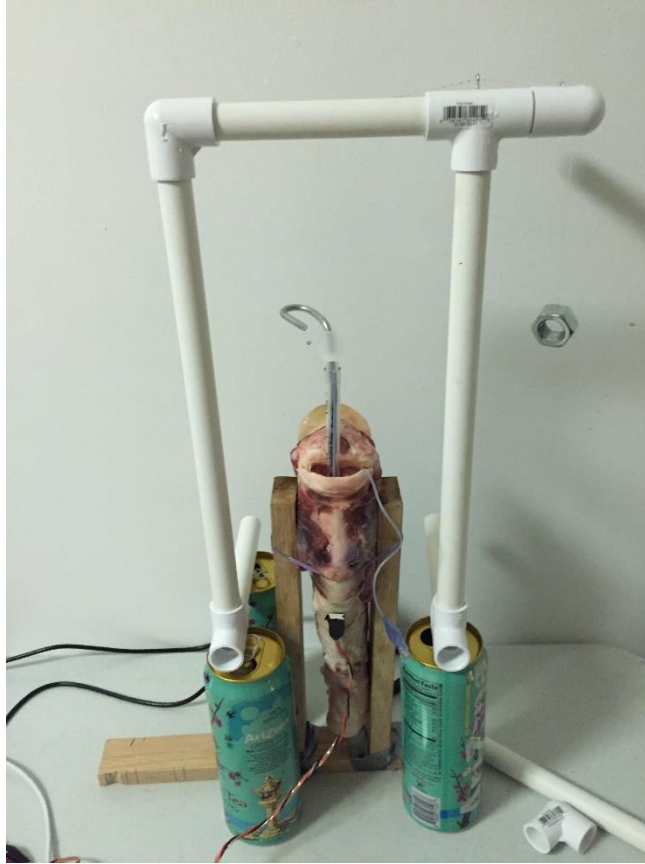
Figure 33. The pig trachea and gantry used to lower an ET tube into the trachea. The gantry system was used as it provided results that are more consistent than previous manual insertion tests. The ET tube is suspended from monofilament wire and held in place with a counter weight. Marks on the wire allow for the tube to be advanced at precise 5mm intervals allowing for more accurate measurements of distance versus output.
