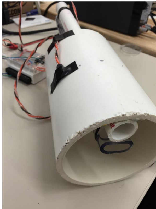
Figure 25. The test setup for evaluating the effects angular displacement has on sensor output. It was theorized that by visualizing the trachea an esophagus from the side would allow for an alternative method of assessing tube placement.
