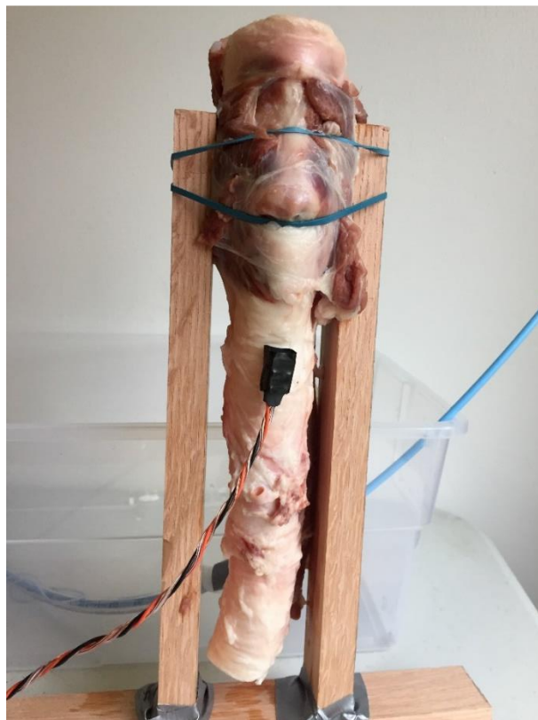
Figure 29. Trachea with the sensor attached. The sensor and foam spacers are held onto the trachea with Cyanoacrylate glue. This glue was chosen as it allows the sensor to be fixed to the trachea without applying pressure on the airway or esophagus.
