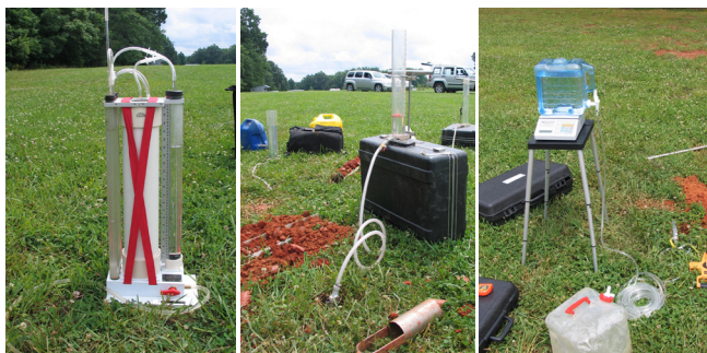
Figure 3. From left, Amoozometer, Johnsonmeter, and Aardvark Permeameter. (Photos by Steven Thomas.)
