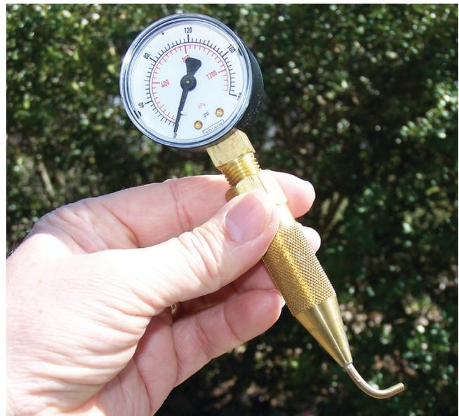
Figure 4. Pitot tube for measuring dynamic or working water pressure at the nozzle. (Photo courtesy of David Ross, University of Maryland.)
