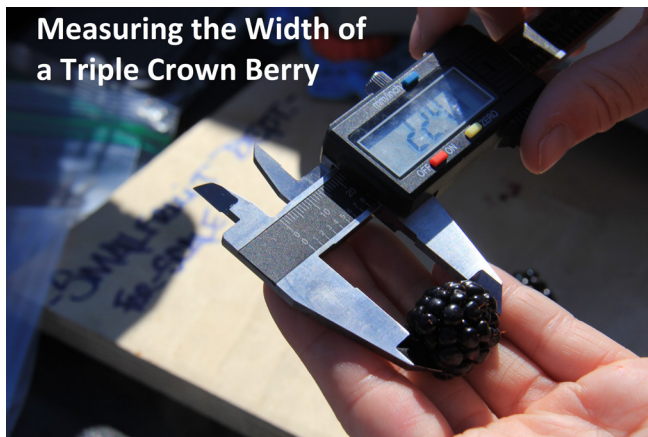
Figure 4. The size of fruit was measured with a vernier caliper scale.
