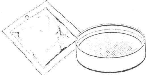
**Alpha-Track Detectors** The alpha-track detector measures radon alpha particle activity. The testing device is made up of a small sheet of special plastic material enclosed in a filtered container (see Figure 3). Radon gas enters the container and radon particles collect on the filter paper. As the gas decays, alpha particles are emitted and permanently mark the plastic sheet.
