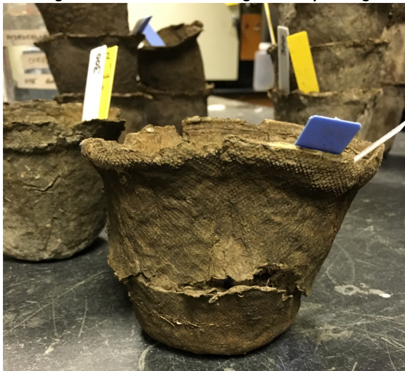
Figure B2-Broken BioPot During Resiliency Testing
