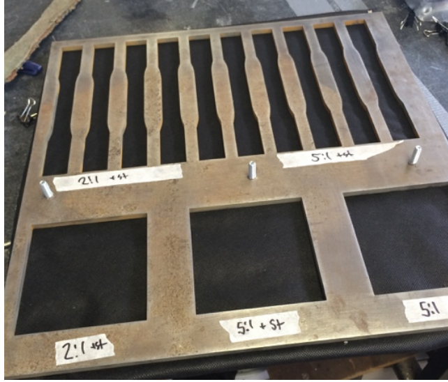
Figure 3-2. Fabricated Stencil Mold Used to Create Coupons for Tensile Testing
