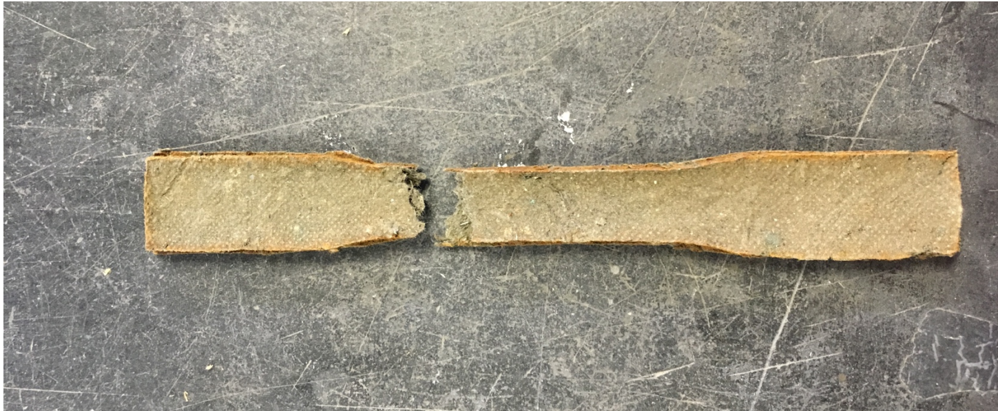
Figure A1- Broken BioPot Coupon
