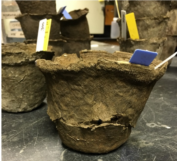
Figure 4-3. Ruptured Biosolids Container
