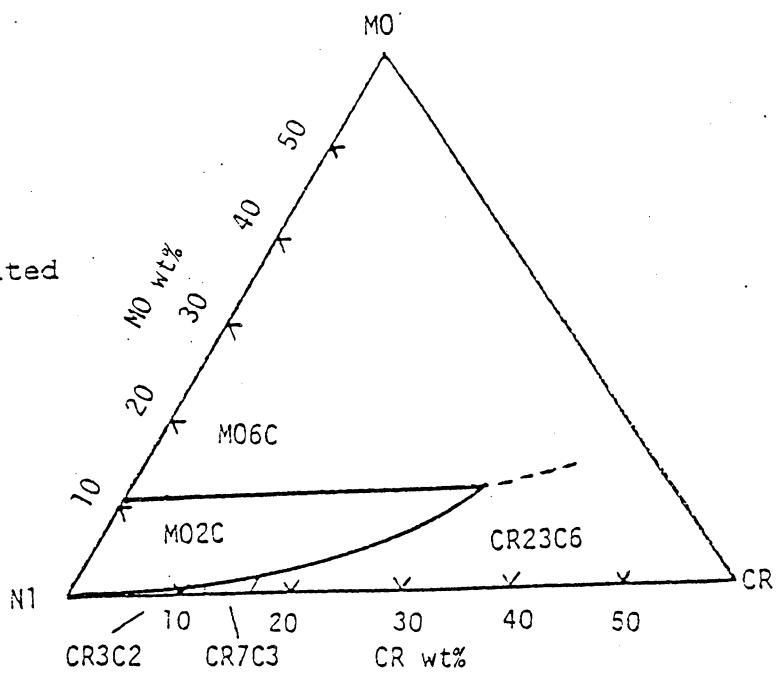
Figure 12. Plot showing stability regions for different carbides. Fig (4) is also shown for comparison.
