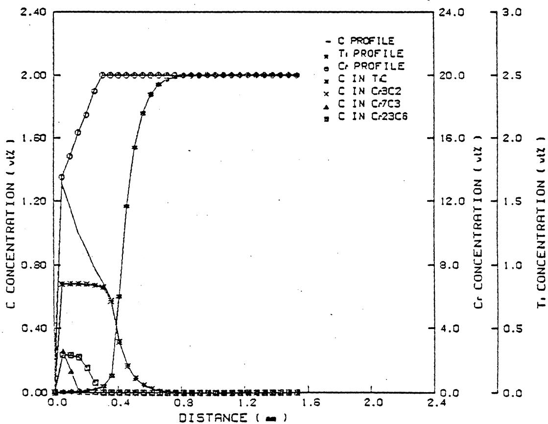
Figure 41. Carburization profiles of Ni-20Cr-2.5Ti alloys, 100 hrs, 850°C, oxidizing condition.
