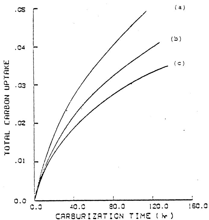
Figure 50. Total carbon uptake as a function of time, oxidizing condition. (a) Ni-30Cr-15Mo, (b) Ni-20Cr-15Mo, (c) Ni-10Cr-15Mo
