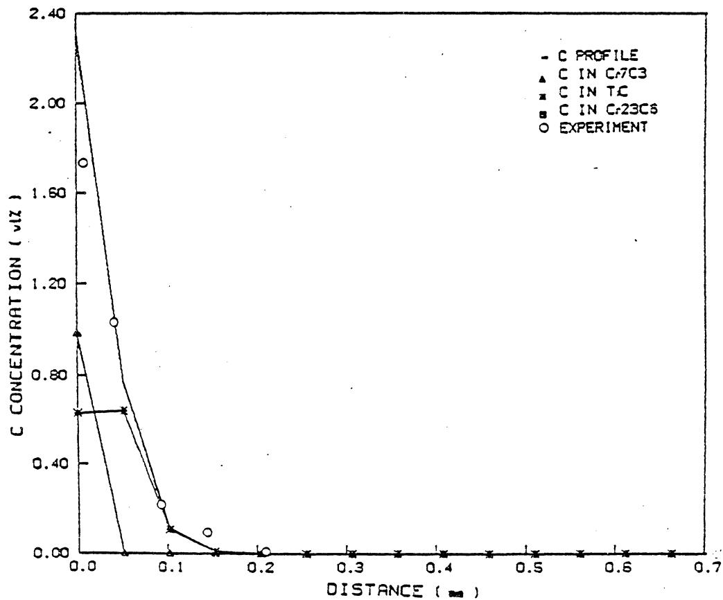
Figure 66. Carburization profile of Inconel X-750, 100hrs
