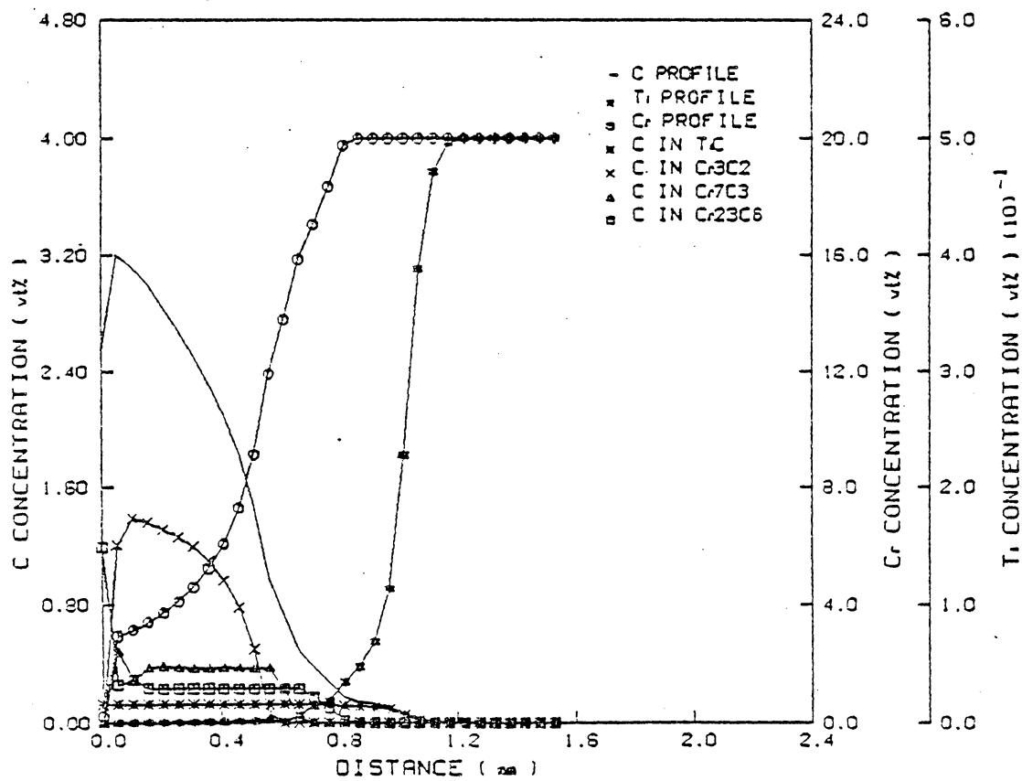
Figure 20. Carburization profiles of Ni-20Cr-.5Ti alloys, 100 hrs, 850°C, non-oxidizing condition.
