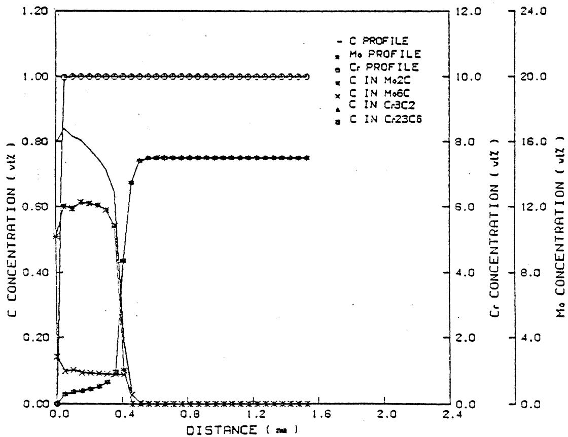
Figure 35. Carburization profiles of Ni-10Cr-15Mo alloys, 100 hrs, 850°C, oxidizing condition.
