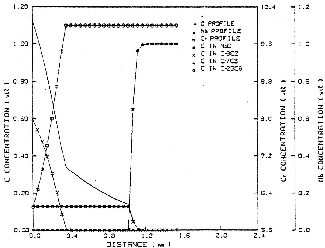
Figure 22. Carburization profiles of Ni-10Cr-1Nb alloys, 100 hrs, 850°C, non-oxidizing condition.
