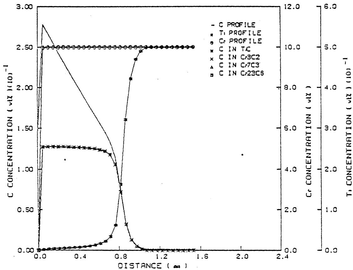
Figure 38. Carburization profiles of Ni-10Cr-.5Ti alloys, 100 hrs, 850°C, oxidizing condition.
