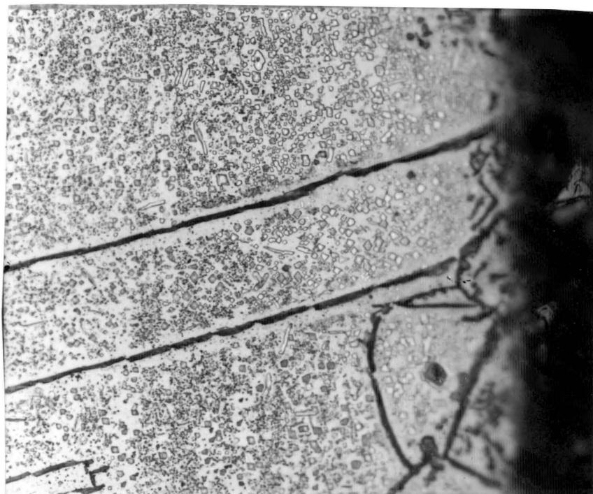
Figure 56. Microstructure showing carbide precipitates in Incoloy 800, 800x, 200hrs.
