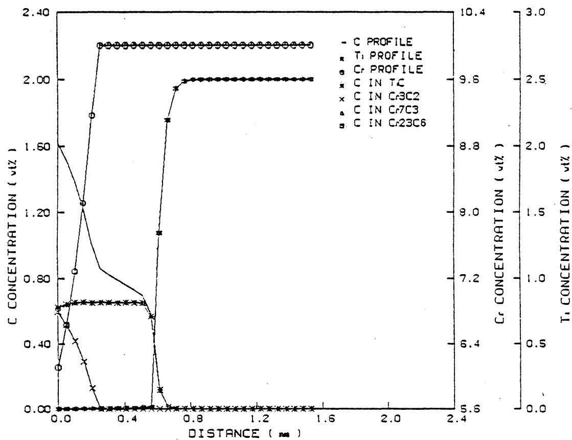
Figure 19. Carburization profiles of Ni-10Cr-2.5Ti alloys, 100 hrs, 850°C, non-oxidizing condition.
