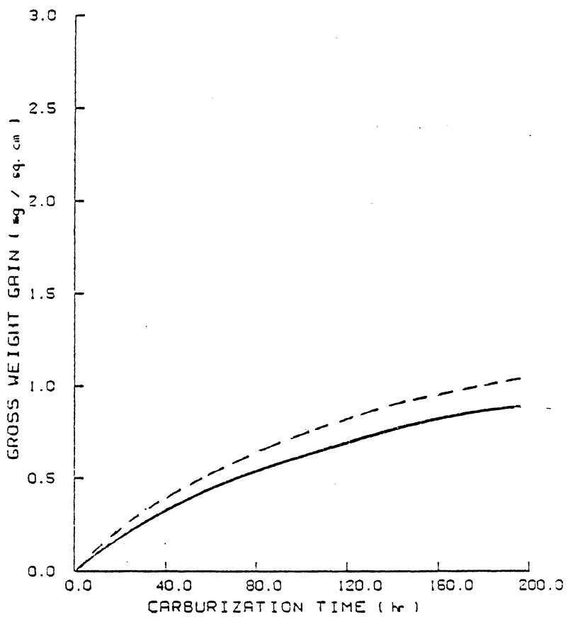
Figure 67. Plot showing calculated and measured weight gains in Inconel K-750. — Measured
