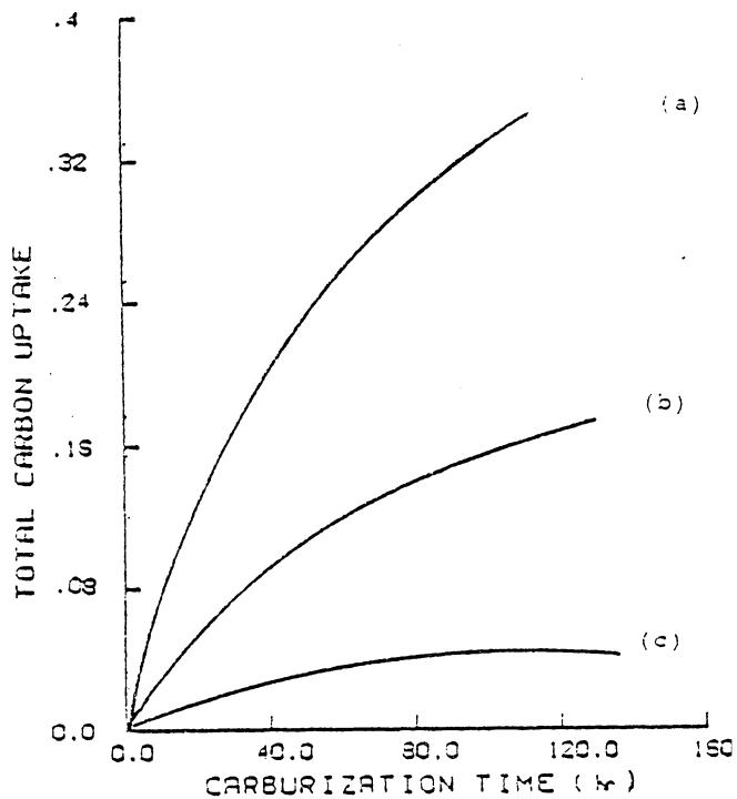
Figure 32. Total carbon uptake as a function of time, non-oxidizing condition. (a) Ni-30Cr-1Nb, (b) Ni-20Cr-1Nb, (c) Ni-10Cr-1Nb
