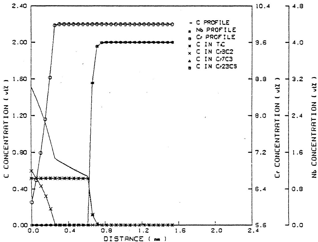
Figure 23. Carburization profiles of Ni-10Cr-4Nb alloys, 100 hrs, 850°C, non-oxidizing condition.
