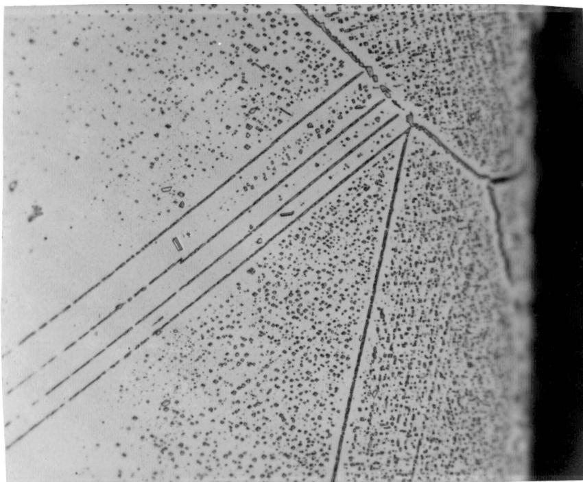
Figure 58. Microstructure showing carbide precipitates
