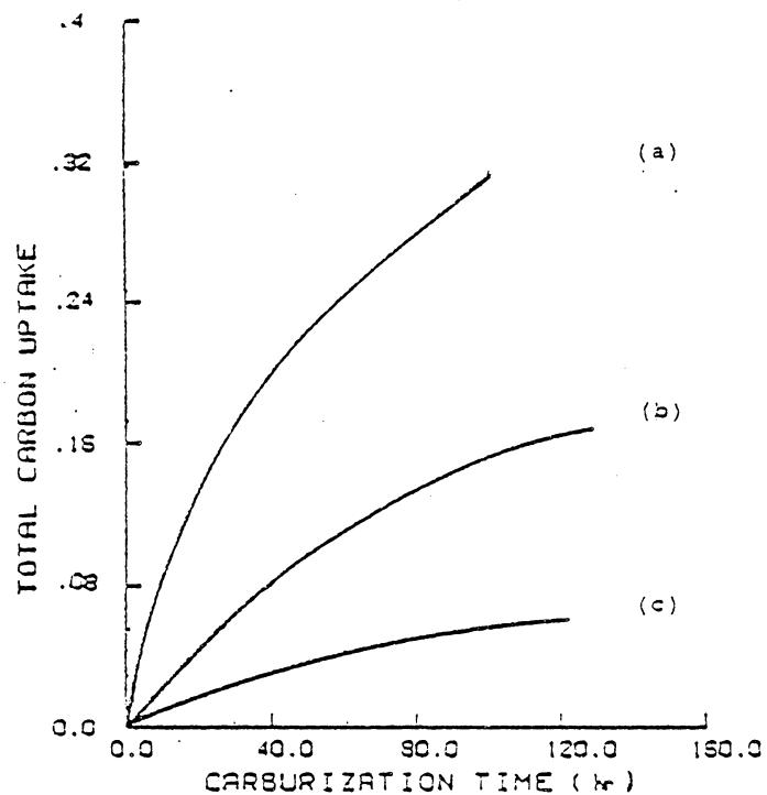
Figure 30. Total carbon uptake as a function of time, non-oxidizing condition. (a) Ni-30Cr-15Mo, (b) Ni-20Cr-15Mo, (c) Ni-10Cr-15Mo
