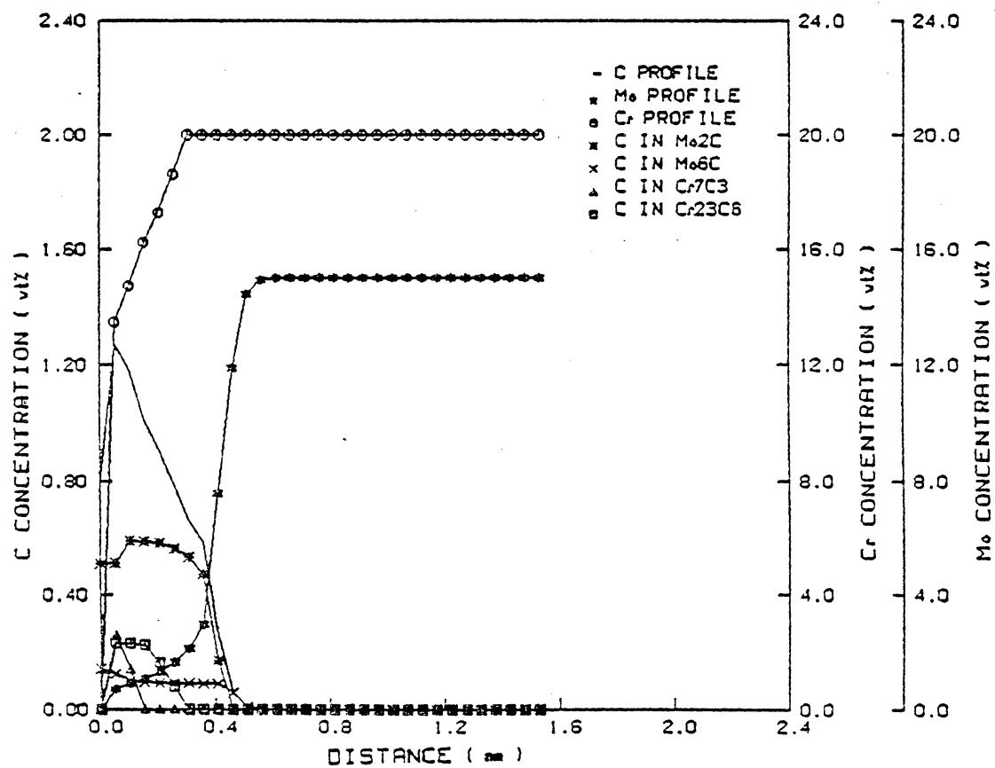
Figure 37. Carburization profiles of Ni-20Cr-15Mo alloys, 100 hrs, 850°C, oxidizing condition.
