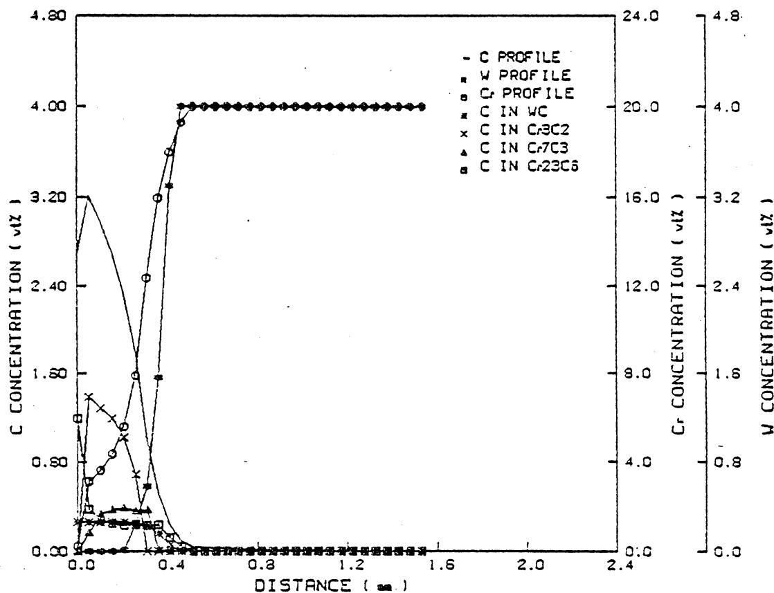
Figure 28. Carburization profiles of Ni-20Cr-4W alloys, 100 hrs, 850°C, non-oxidizing condition.
