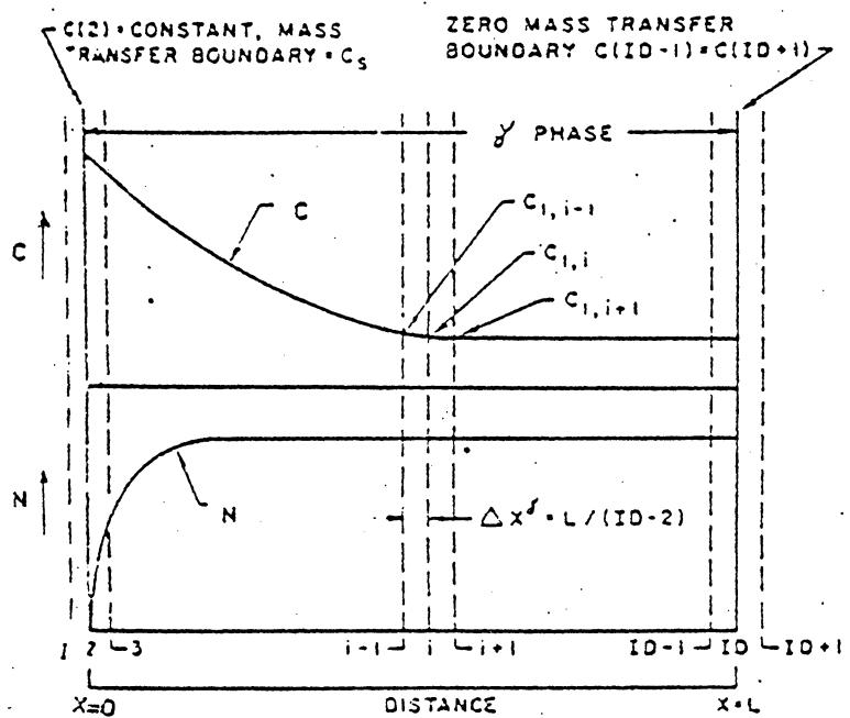
Figure 11. Schematic diagram of the space-composition grid for the numerical model of carburization.
