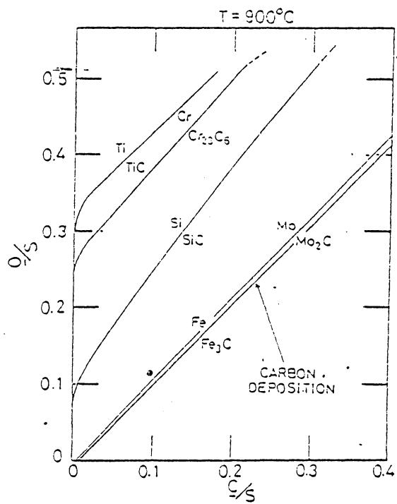
Figure 6. Equilibrium lines between metals and metal carbides at 900°C as function of atomic fraction of oxygen (O/S), and carbon (C/S).
