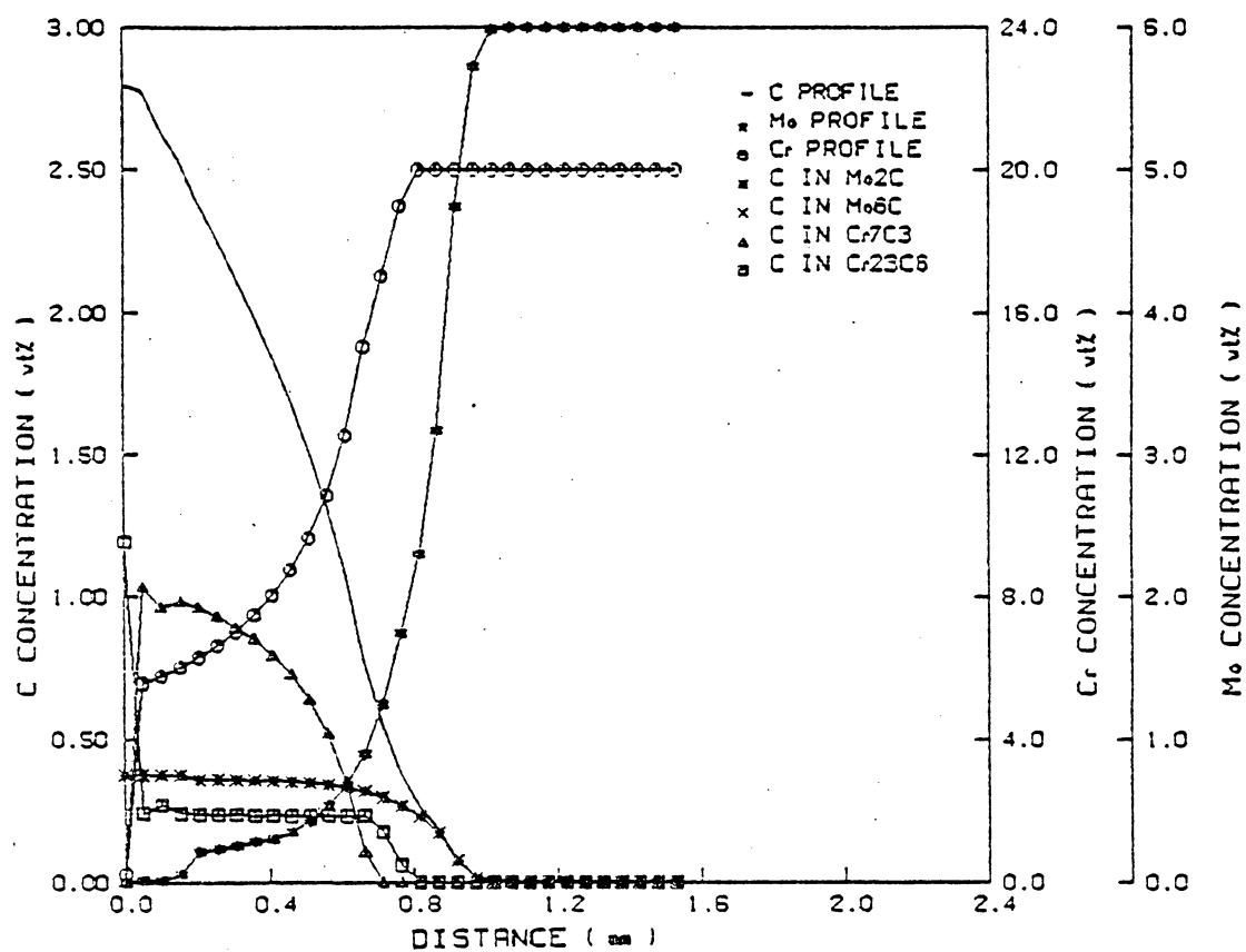
Figure 16. Carburization profiles of Ni-20Cr-6Mo alloys, 100 hrs, 850°C, non-oxidizing condition.
