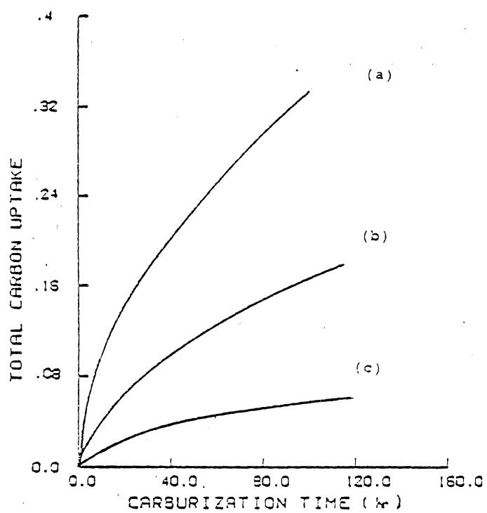
Figure 31. Total carbon uptake as a function of time, non-oxidizing condition. (a) Ni-30Cr-2.5Ti, (b) Ni-20Cr-2.5Ti, (c) Ni-10Cr-2.5Ti
