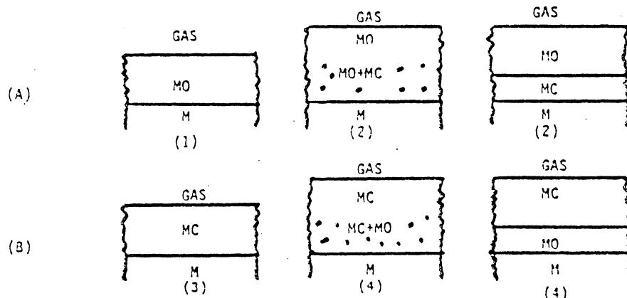
Figure 3. M-C-O phase stability and effect of gas composition and reaction paths on surface scales.
