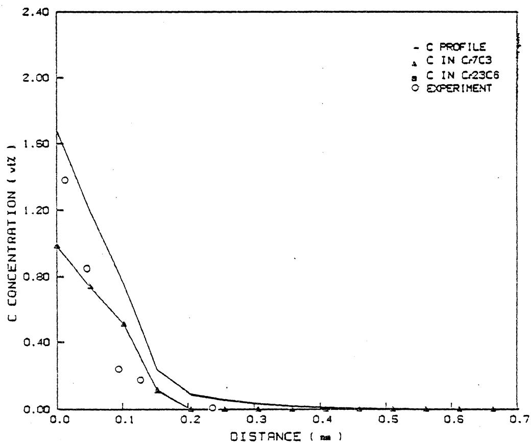
Figure 65. Carburization profile of Inconel 600, 200hrs
