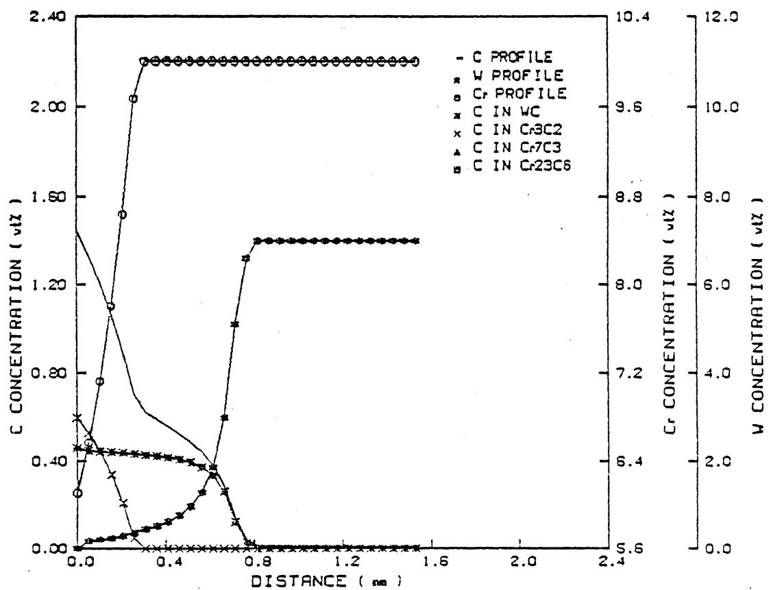
Figure 27. Carburization profiles of Ni-10Cr-7W alloys, 100 hrs, 850°C, non-oxidizing condition.
