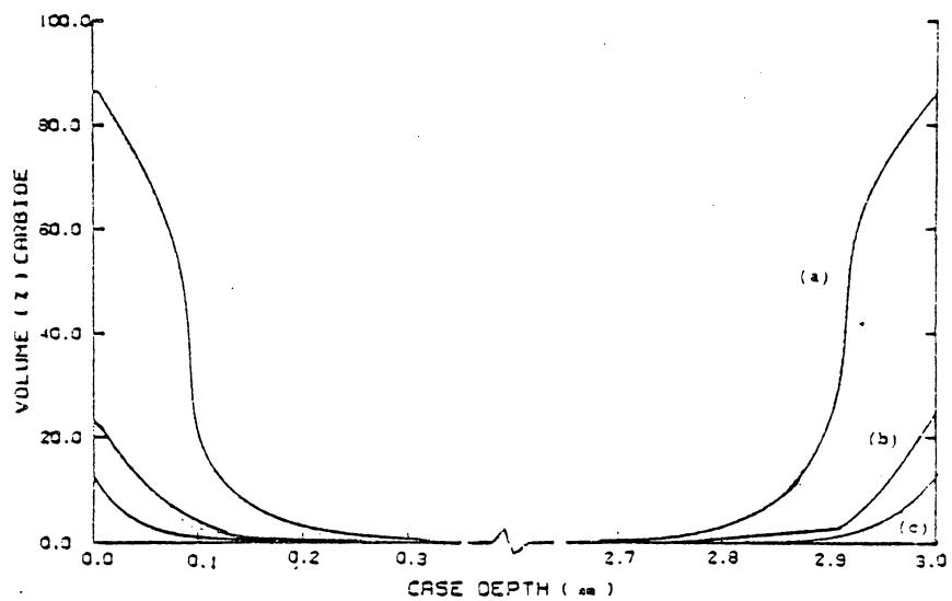
Figure 63. Plot showing amount of carbide present as a function of penetration distance for 200 hrs.
