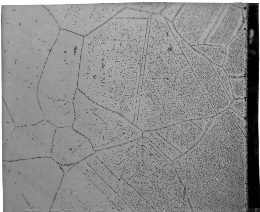
Figure 59. Microstructure showing carbide precipitates in Inconel 601, 400x, 200Hrs.
