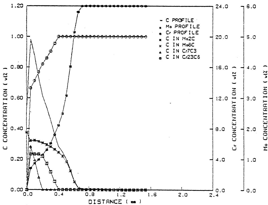
Figure 36. Carburization profiles of Ni-20Cr-6Mo alloys, 100 hrs, 850°C, oxidizing condition.
