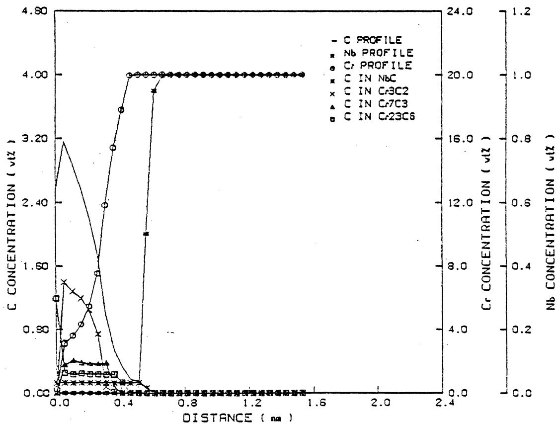
Figure 24. Carburization profiles of Ni-20Cr-1Nb alloys, 100 hrs, 850°C, non-oxidizing condition.
