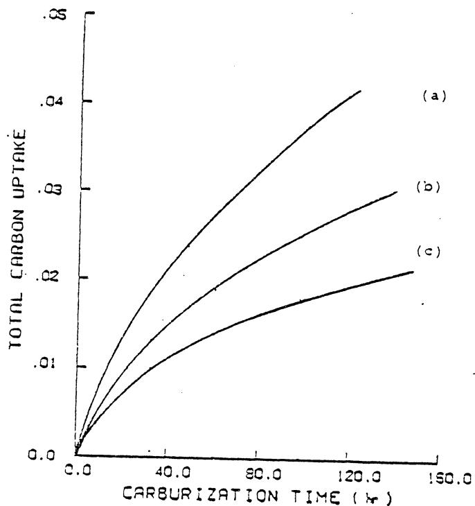
Figure 53. Total carbon uptake as a function of time, oxidizing condition. (a) Ni-30Cr-4W, (b) Ni-20Cr-4W, (c) Ni-10Cr-4W
