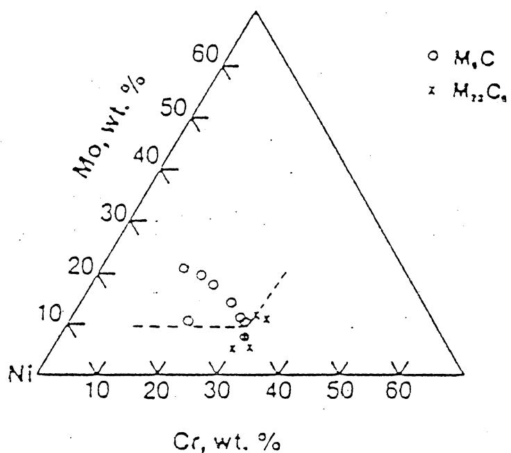
Figure 4. Plot showing the austenite compositions of alloys and the type of carbide.
