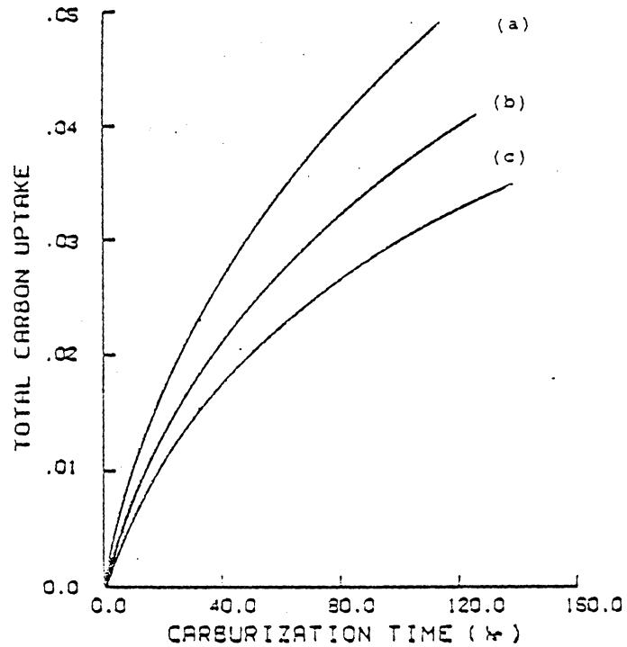
Figure 51. Total carbon uptake as a function of time, oxidizing condition. (a) Ni-30Cr-2.5Ti, (b) Ni-20Cr-2.5Ti, (c) Ni-10Cr-2.5Ti
