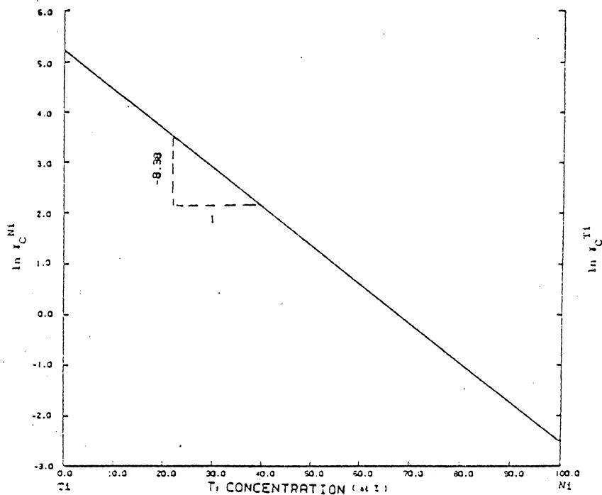
Figure 13. plot for calculation of interaction parameter  $e_{12}$ .
