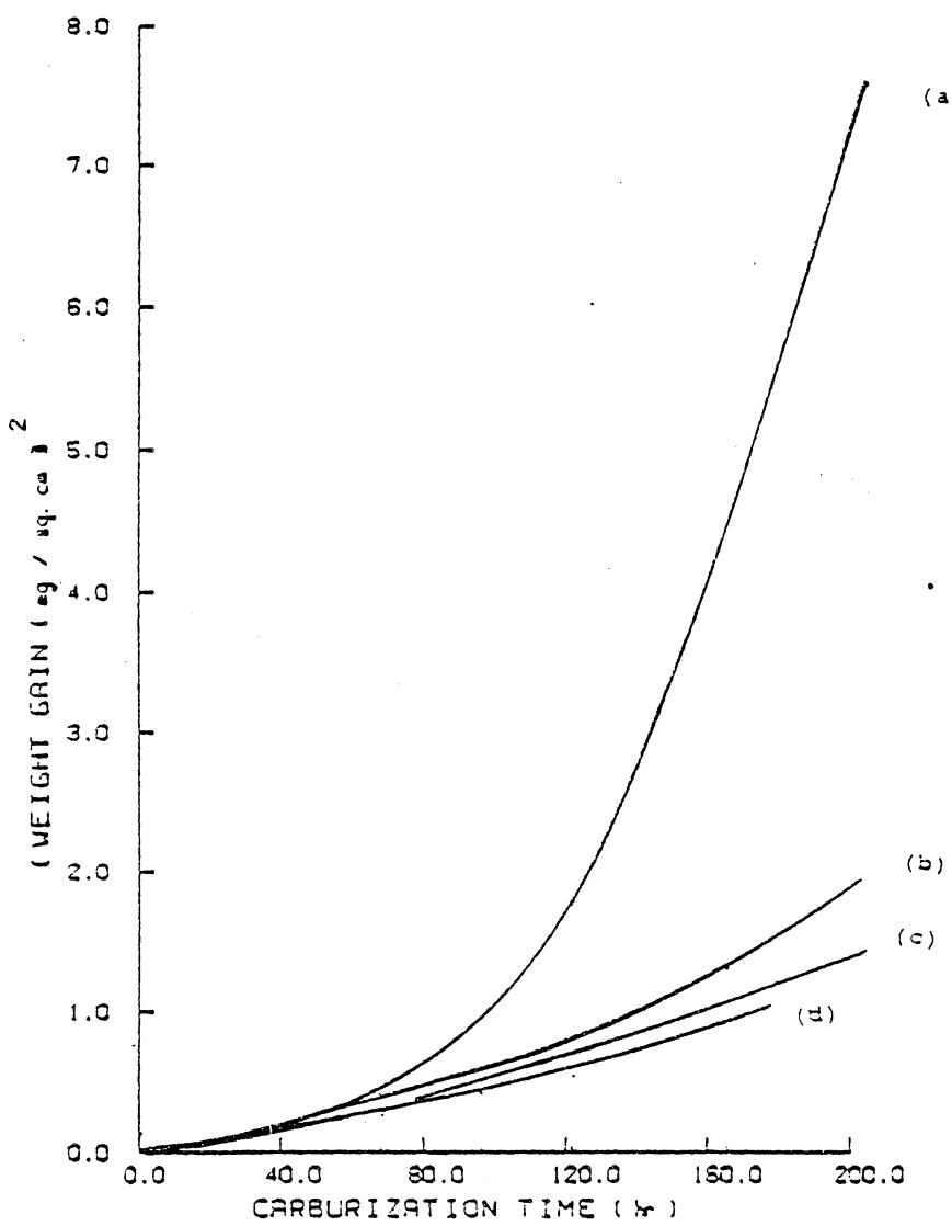
Figure 64. Relationship between the square of the weight gain and time.
