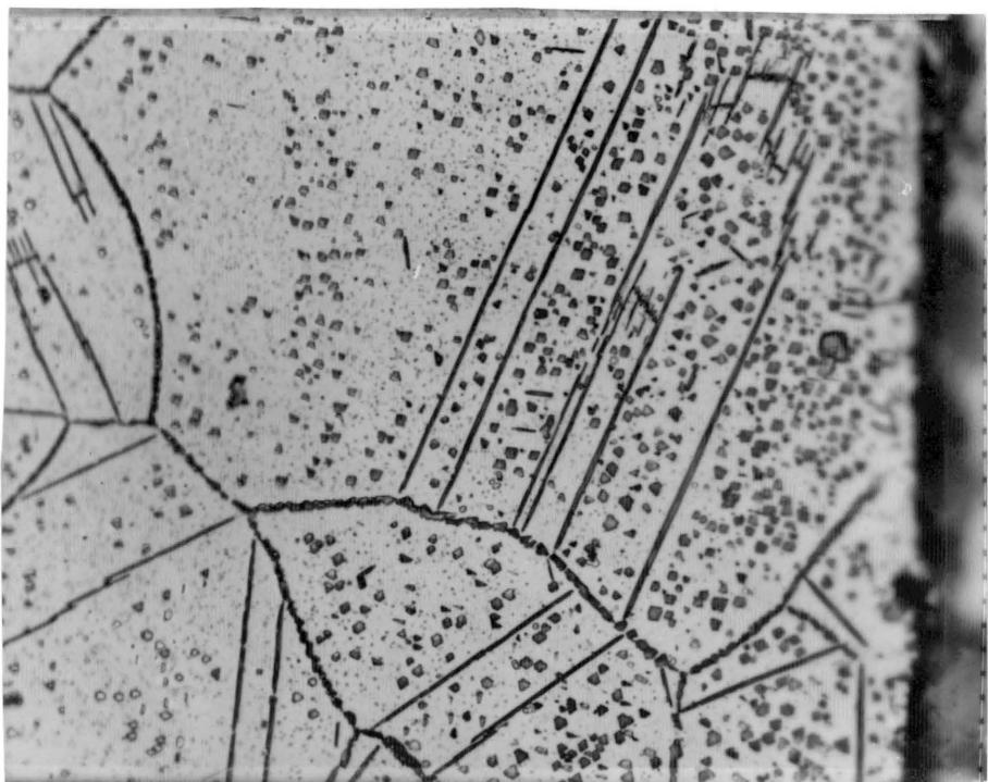
Figure 55. Microstructure showing carbide precipitates in Incoloy 800, 800x, 100Hrs.
