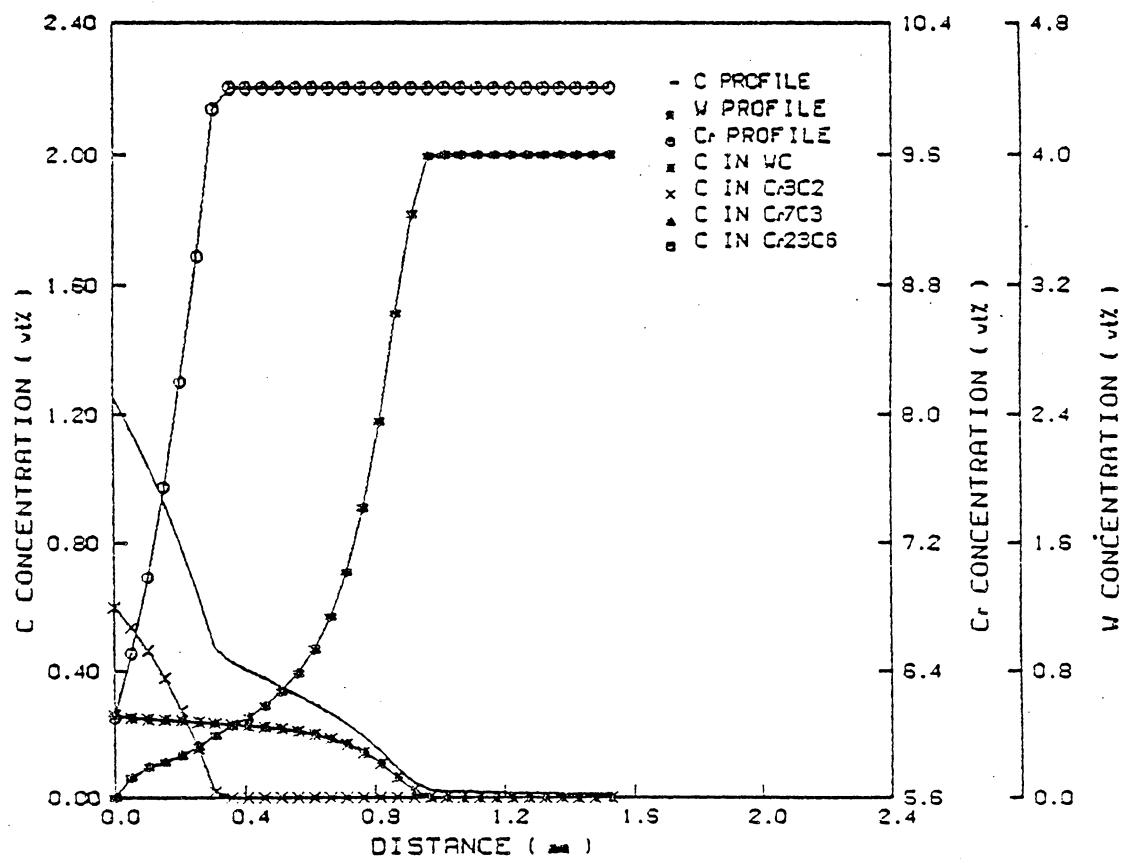
Figure 26. Carburization profiles of Ni-10Cr-4W alloys, 100 hrs, 850°C, non-oxidizing condition.
