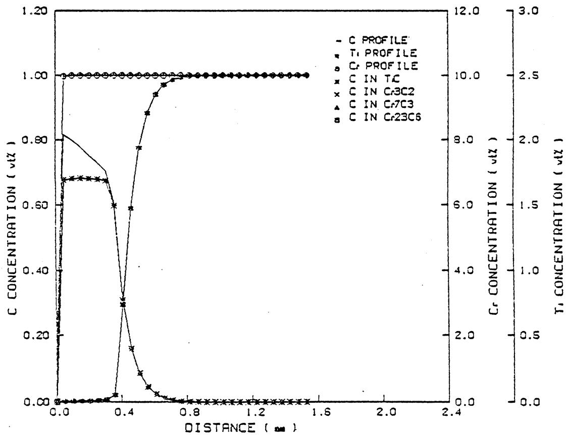
Figure 39. Carburization profiles of Ni-10Cr-2.5Ti alloys, 100 hrs, 850°C, oxidizing condition.
