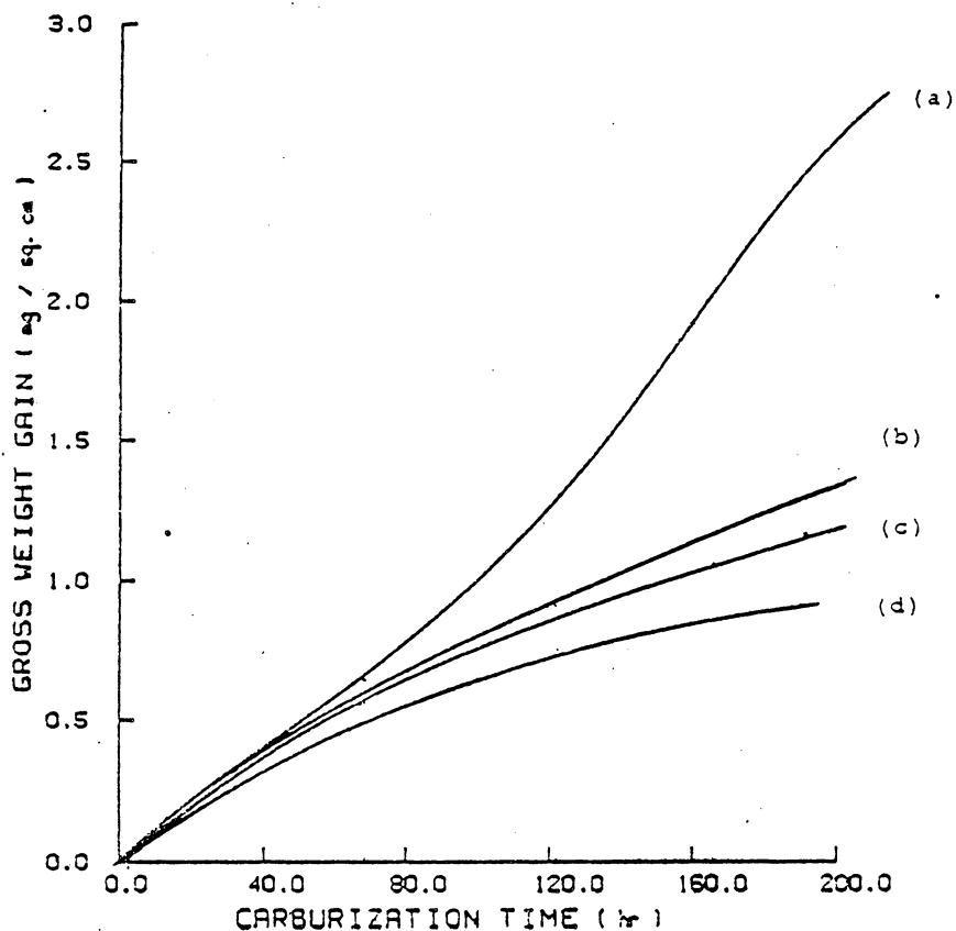
Figure 61. Weight gain determinations for the alloys exposed to  $H_2\text{-CH}_4$  environment of 1.0 carbon activity at 850°C. (a) Incoloy 800, (b) Inconel 600, (c) Inconel 601, (d) Inconel X-750.
