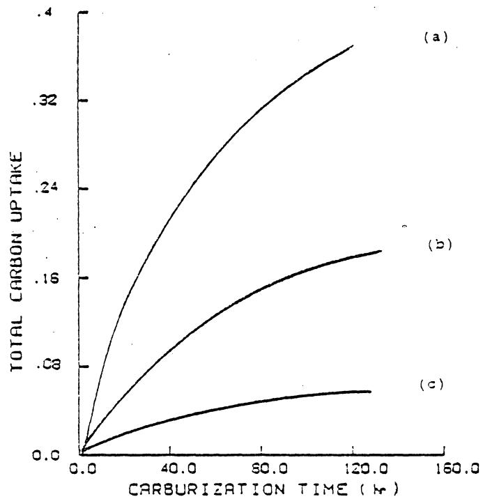
Figure 33. Total carbon uptake as a function of time, non-oxidizing condition. (a) Ni-30Cr-4W, (b) Ni-20Cr-4W, (c) Ni-10Cr-4W
