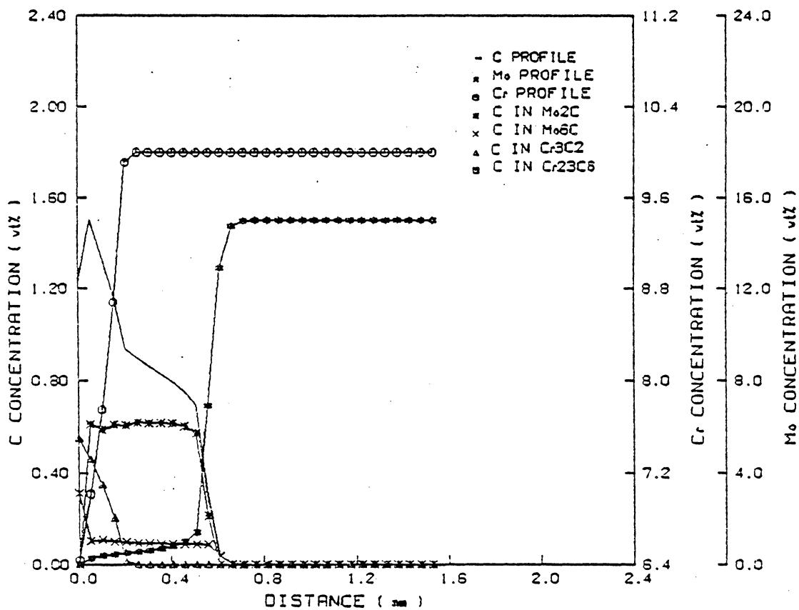
Figure 15. Carburization profiles of Ni-10Cr-15Mo alloys, 100 hrs, 650°C, non-oxidizing condition.
