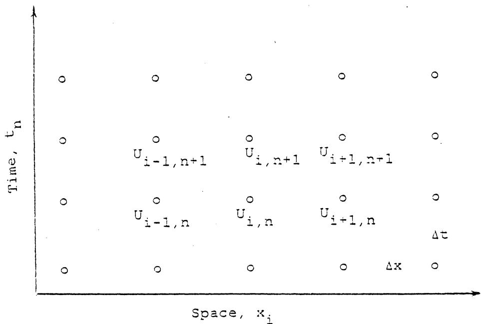
Figure 10. Grid spacing for finite difference model.
