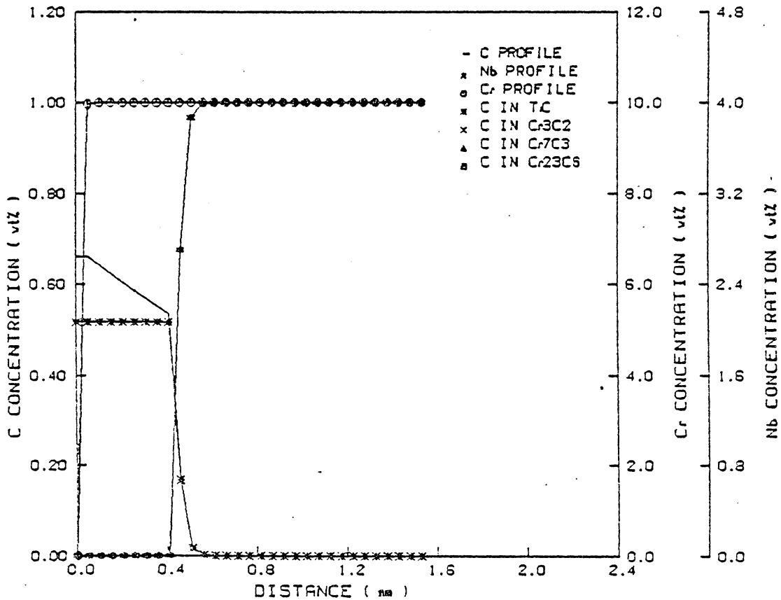
Figure 43. Carburization profiles of Ni-10Cr-4Nb alloys, 100 hrs, 850°C, oxidizing condition.
