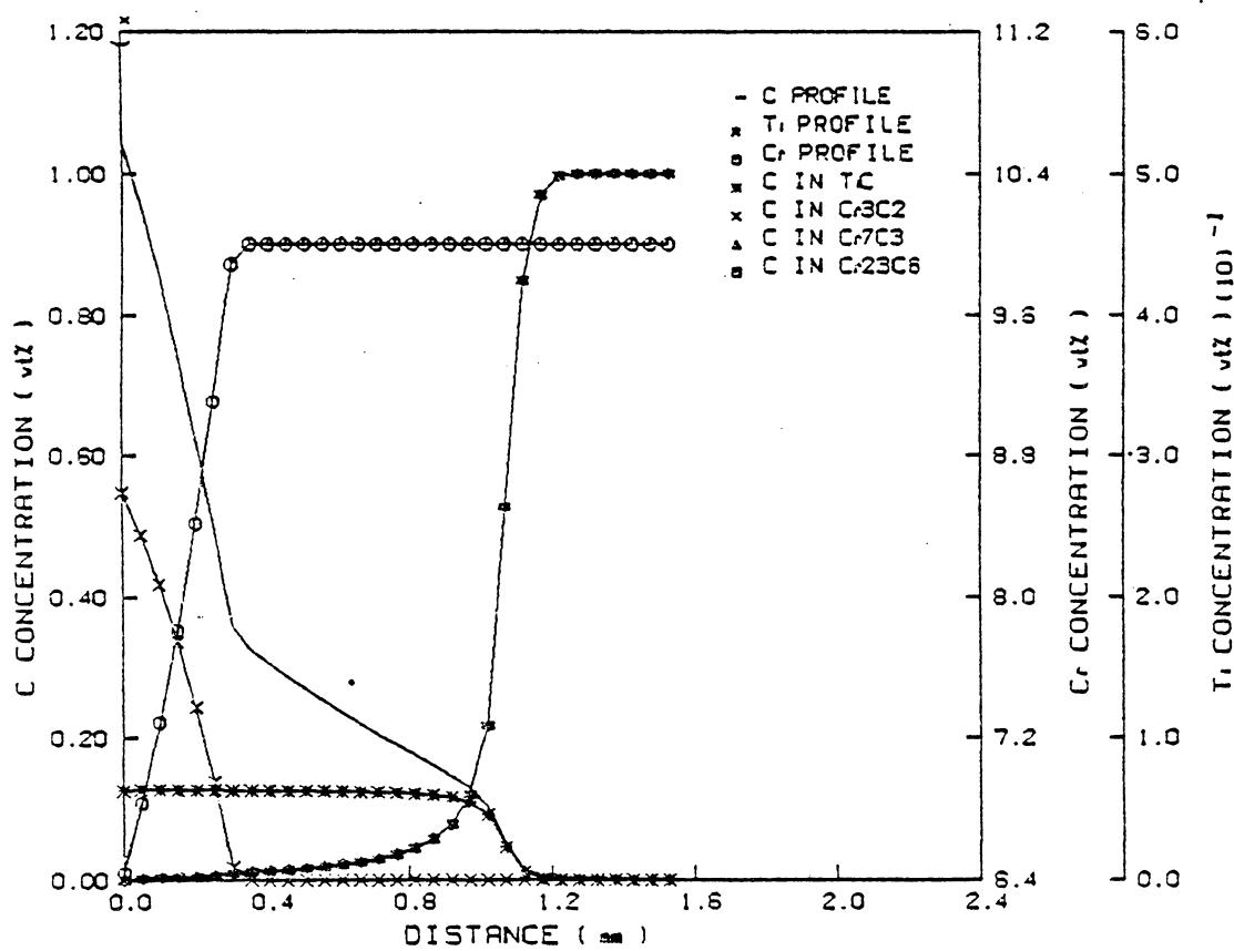
Figure 18. Carburization profiles of Ni-10Cr-.5Ti alloys, 100 hrs, 850°C, non-oxidizing condition.
