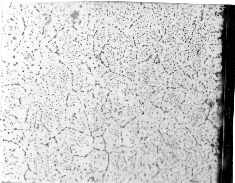
Figure 57. Microstructure showing carbide precipitates in Inconel 600, 800x, 200hrs.
