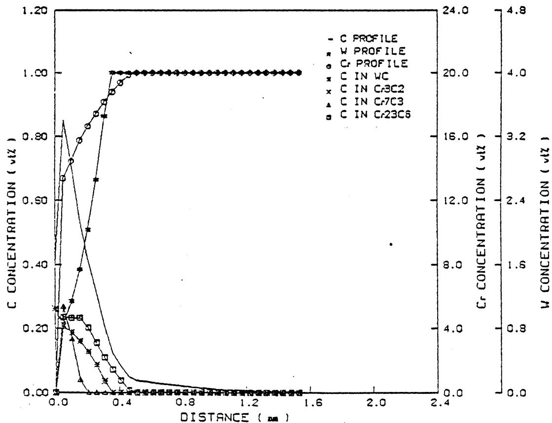
Figure 48. Carburization profiles of Ni-20Cr-4W alloys, 100 hrs, 850°C, oxidizing condition.
