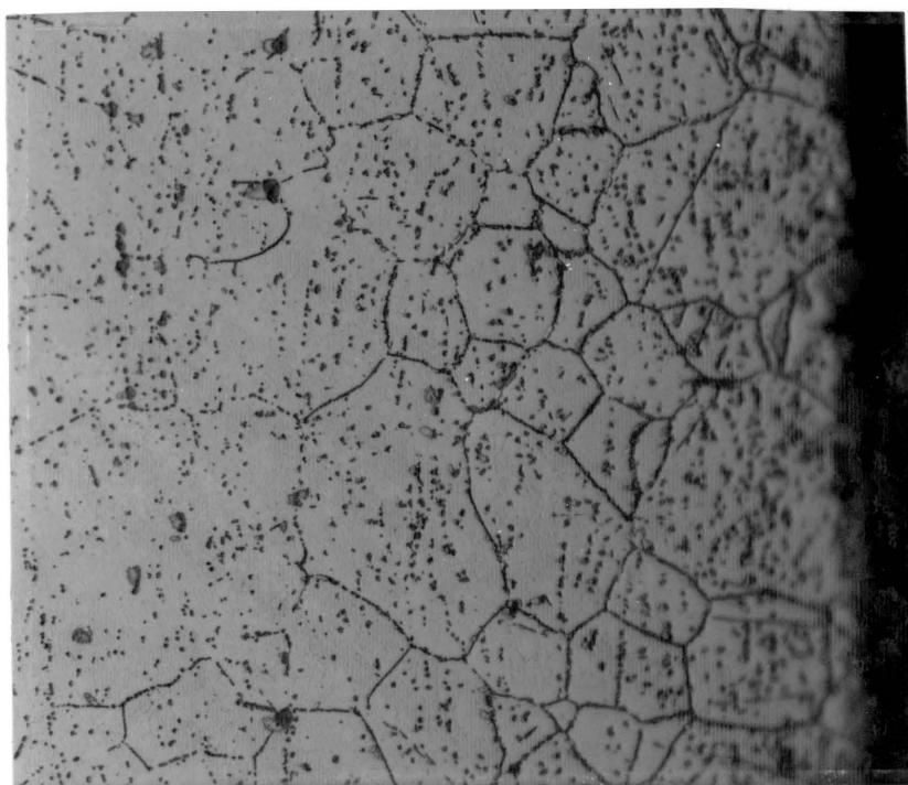
Figure 60. Microstructure showing carbide precipitates in Inconel X-750, 625x, 100hrs.
