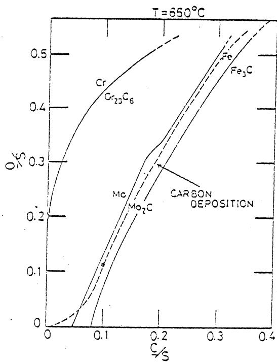
Figure 5. Equilibrium lines between metals and metal carbides at  $650^\circ\text{C}$  as function of atomic fraction of oxygen ( $\text{O/S}$ ), and carbon ( $\text{C/S}$ ).
