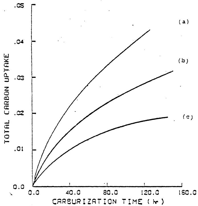
Figure 52. Total carbon uptake as a function of time, oxidizing condition. (a) Ni-30Cr-1Nb, (b) Ni-20Cr-1Nb, (c) Ni-10Cr-1Nb
