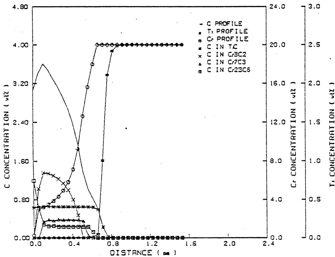
Figure 21. Carburization profiles of Ni-20Cr-2.5Ti alloys, 100 hrs, 850°C, non-oxidizing condition.
