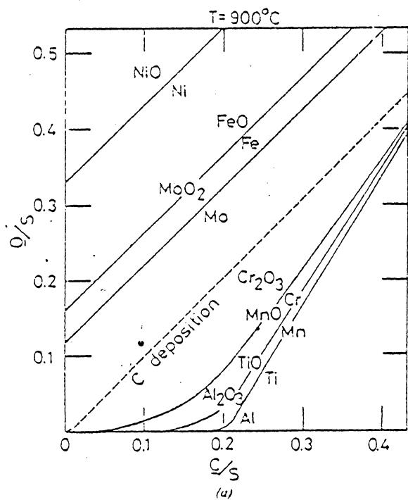
Figure 7. Equilibrium lines between metals and metal oxides at 900°C as function of atomic fraction of oxygen (O/S), and carbon (C/S).
