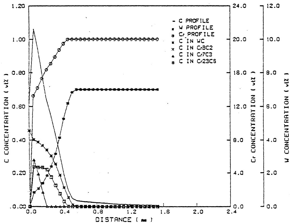
Figure 49. Carburization profiles of Ni-20Cr-7W alloys, 100 hrs, 850°C, oxidizing condition.
