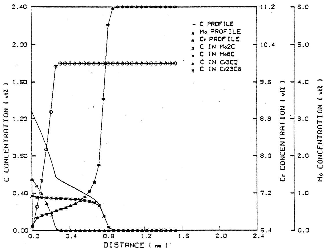
Figure 14. Carburization profiles of Ni-10Cr-6Mo alloys, 100 hrs, 850°C, non-oxidizing condition
