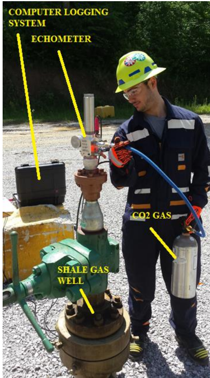
Figure 27: User Charging the Echometer for an Acoustic Test
