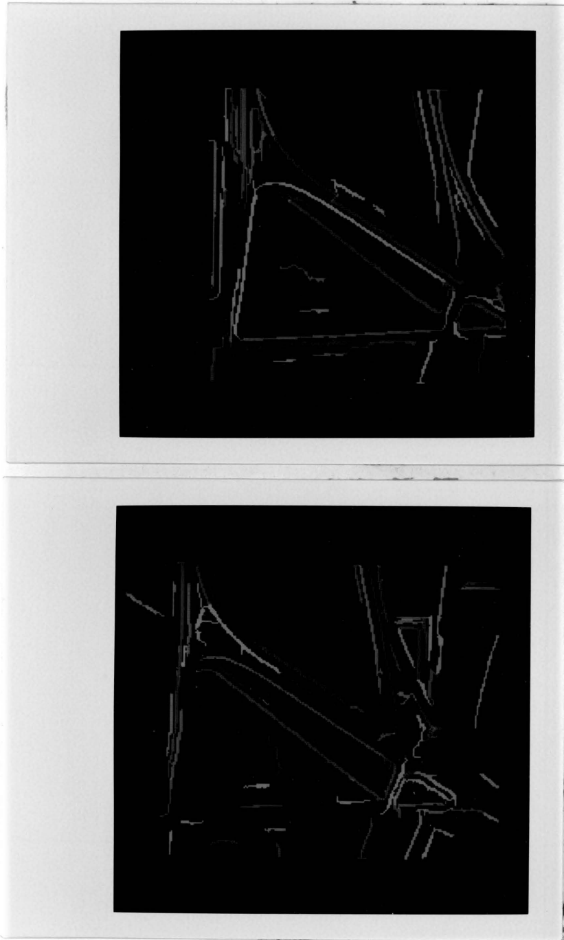
Figure 36: Arc segments extracted from the images of Figure 35.
