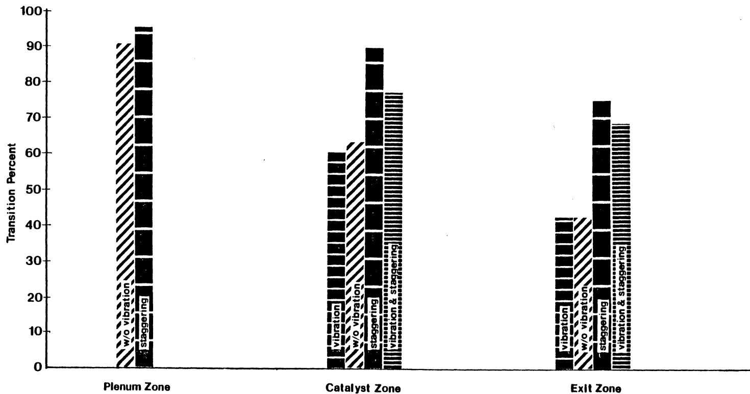
Figure 5.39. A Summary of Percent Gas-Transition Completion in the Cold-Flow Micro-reactor 2.4 Seconds After the Initial Detector Response. Shown Is the Argon-to-Helium Feed Transition at 417 Actual \text{mm}^3/\text{s} .
