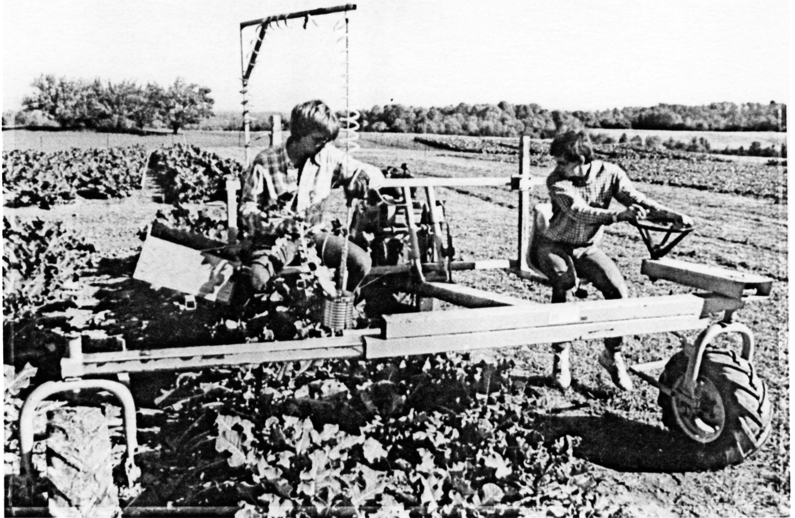
Figure 20. Vegetable harvesting aid with the cutting device operated from the seated position.
