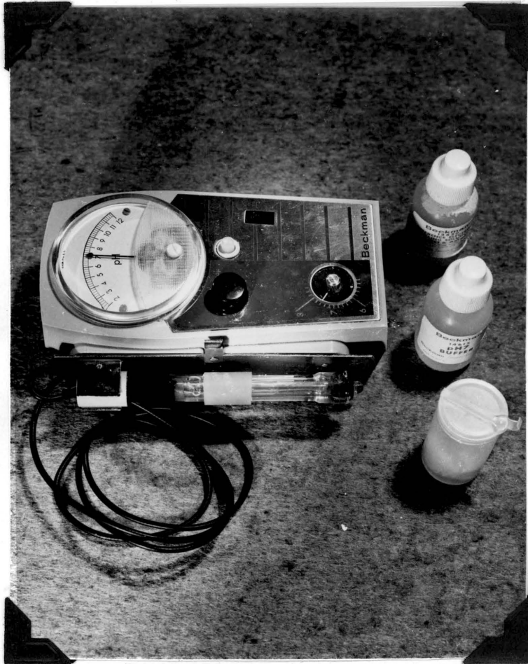
FIG. 4. THE pH METER.
