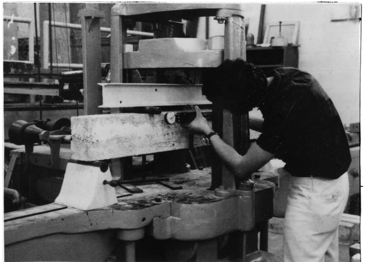
Figure 8. Measuring Strains with the Whittemore Strain Gage.
