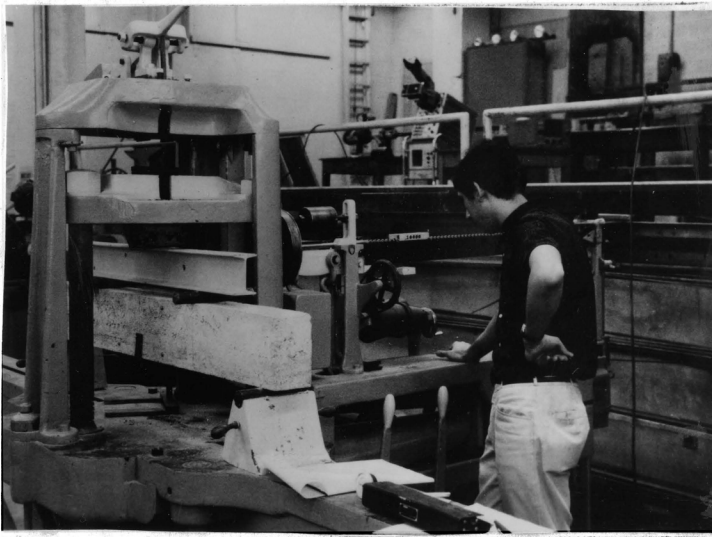
Figure 7. Applying Load to a Beam.
