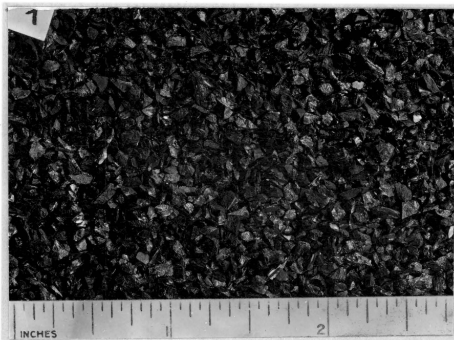
Coal Sample No. 7, High Volatile Bituminous A, Stonega Coke and Coal Co., Big Stone Gap, Virginia.
