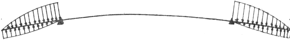
Fig. 18-b Corrective Loading Scheme on The Cantilever
