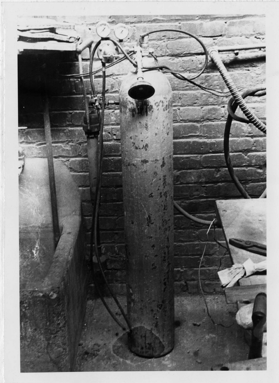
CO 2 Gassing Unit
