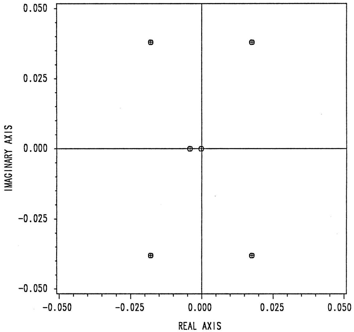
Figure 18. Eigenvalues of Linearized System with  $\mu = 320 \text{ sec/lb}$
