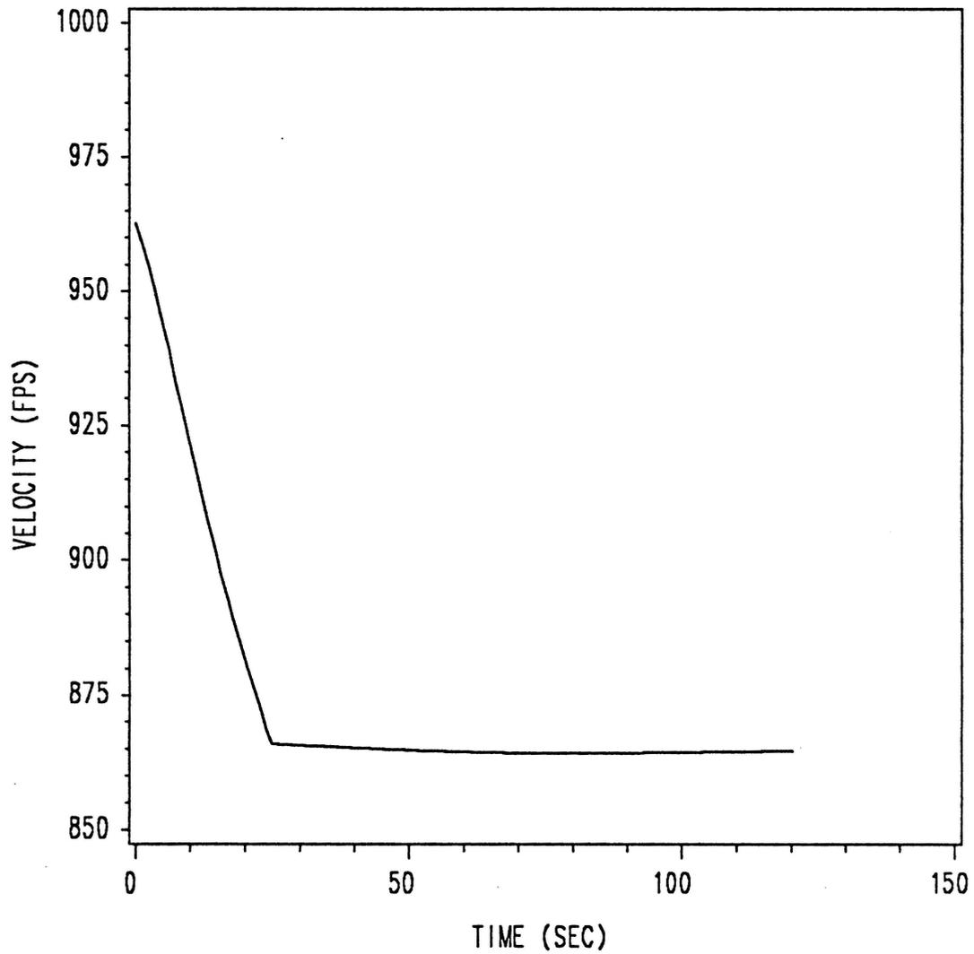
Figure 32. Velocity Time History for (Zero)Bang-Singular Control
