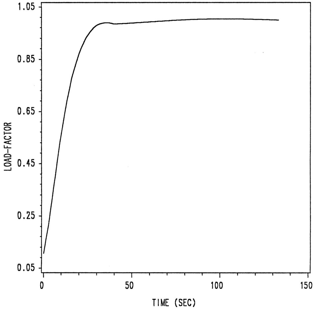
Figure 29. Load-Factor Time History for (Full)Bang-Singular Control
