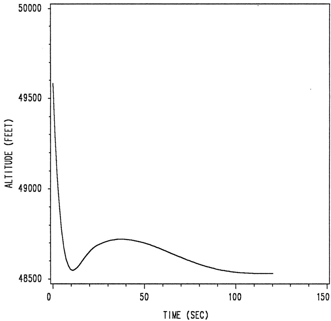
Figure 30. Altitude Time History for (Zero)Bang-Singular Control
