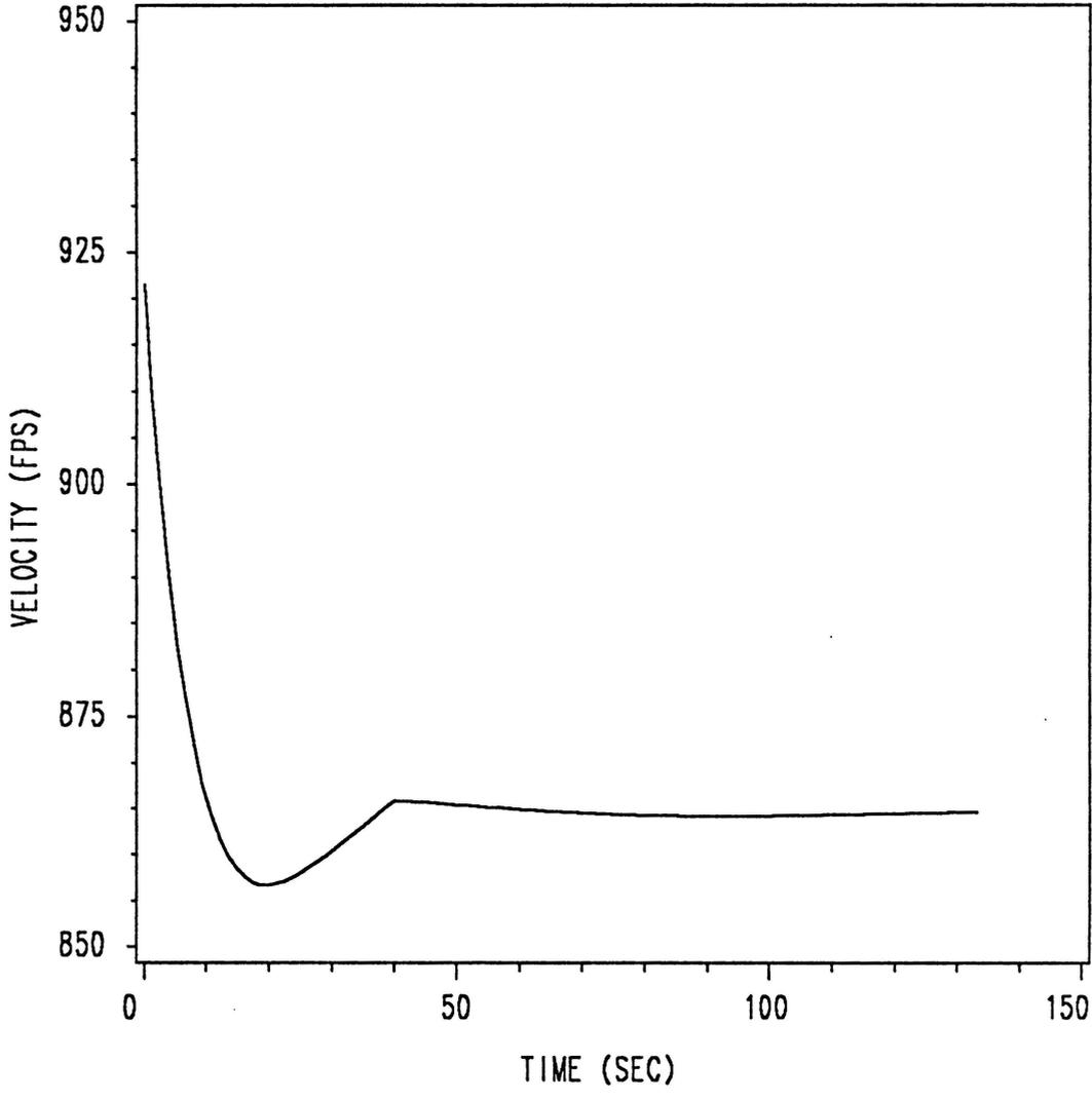
Figure 27. Velocity Time History for (Full)Bang-Singular Control
