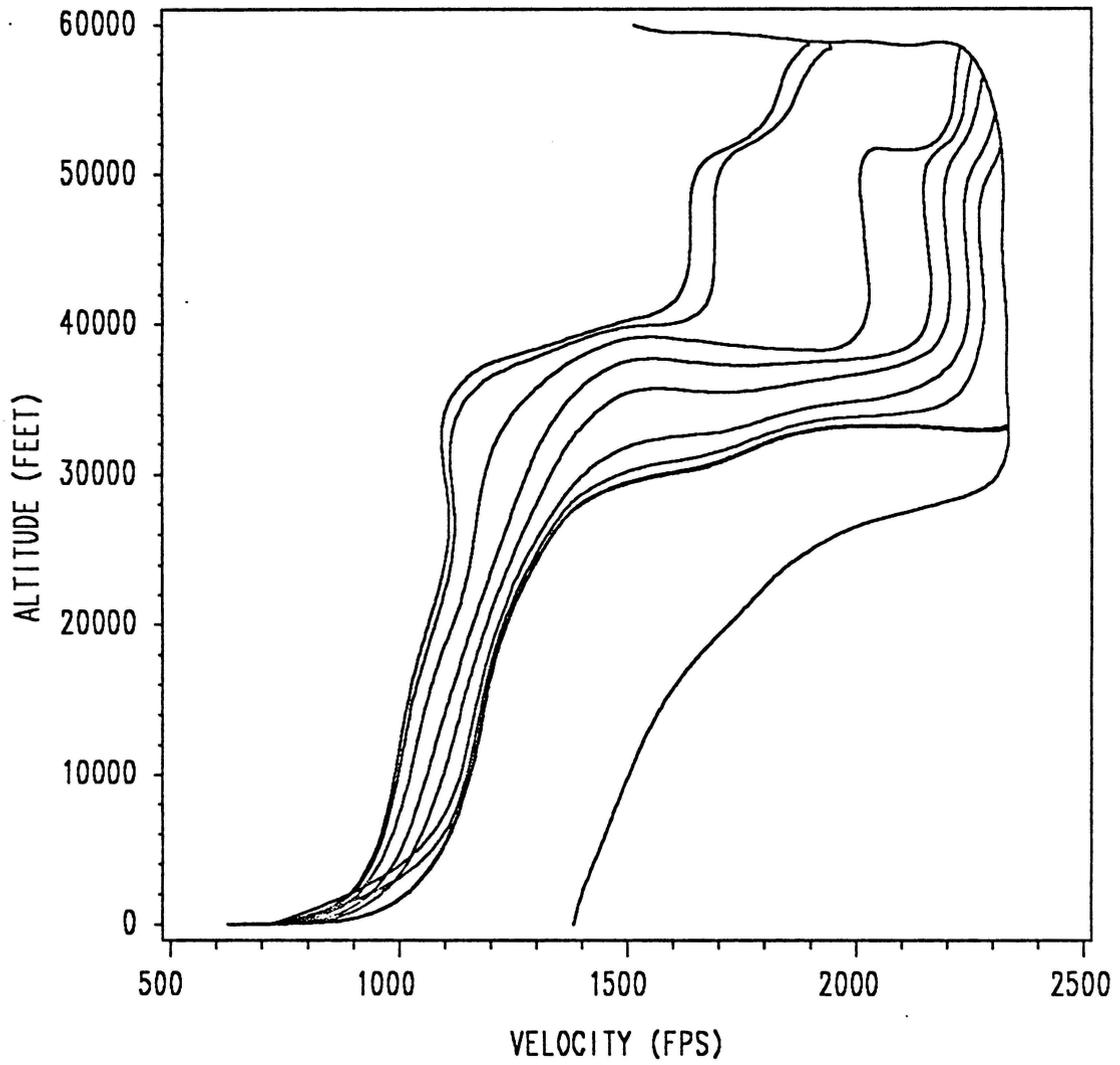
Figure 16. Full-Throttle Cruise-Dash Trajectories in the (h,V) Plane
