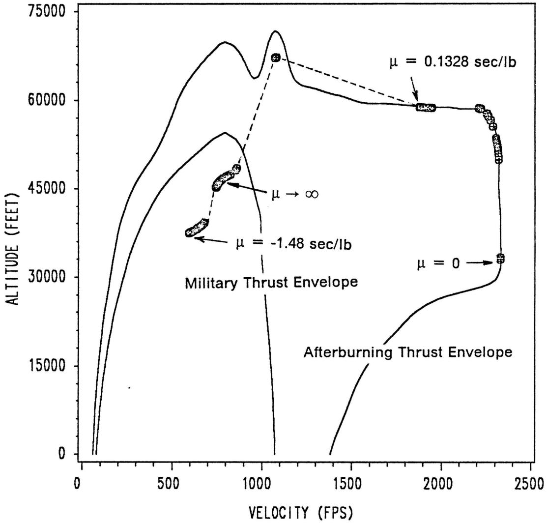
Figure 1. Cruise-Dash Points in the (h,V) Plane
