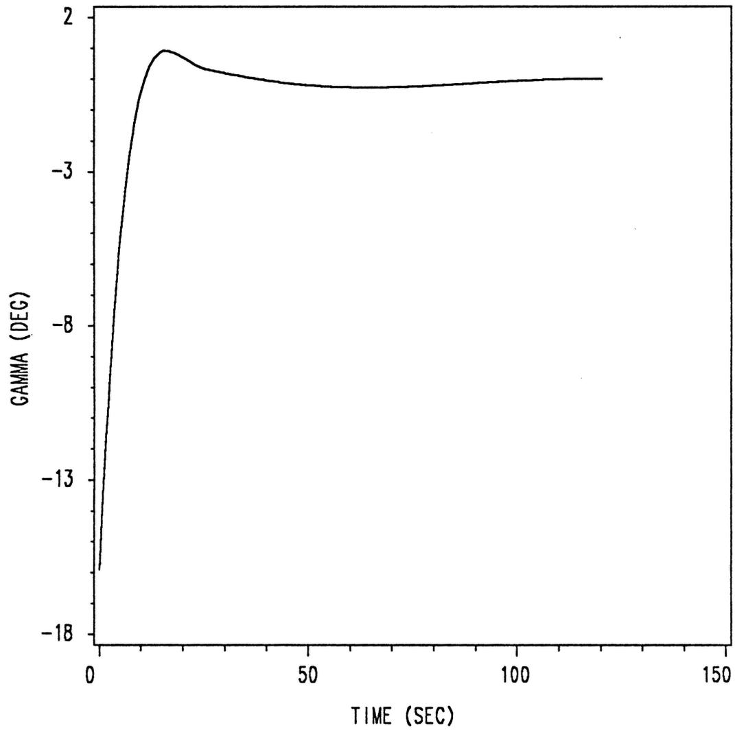
Figure 31. Path-Angle Time History for (Zero)Bang-Singular Control
