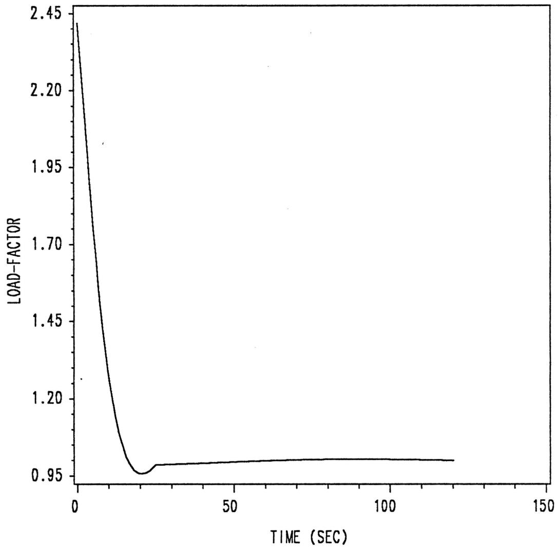
Figure 34. Load-Factor Time History for (Zero)Bang-Singular Control
