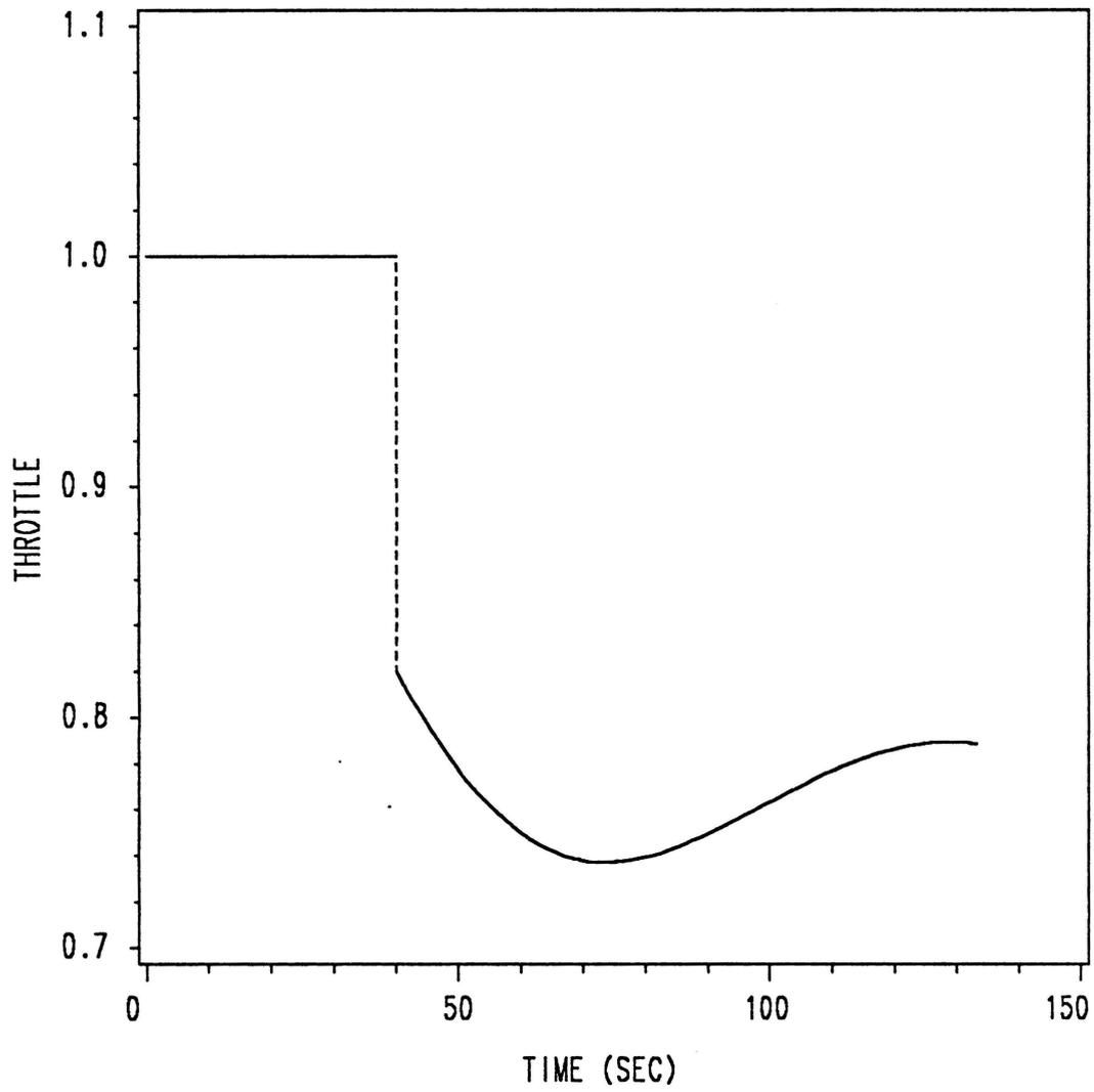
Figure 28. Throttle Time History for (Full)Bang-Singular Control
