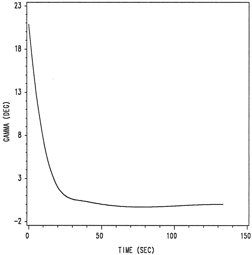
Figure 26. Path-Angle Time History for (Full)Bang-Singular Control
