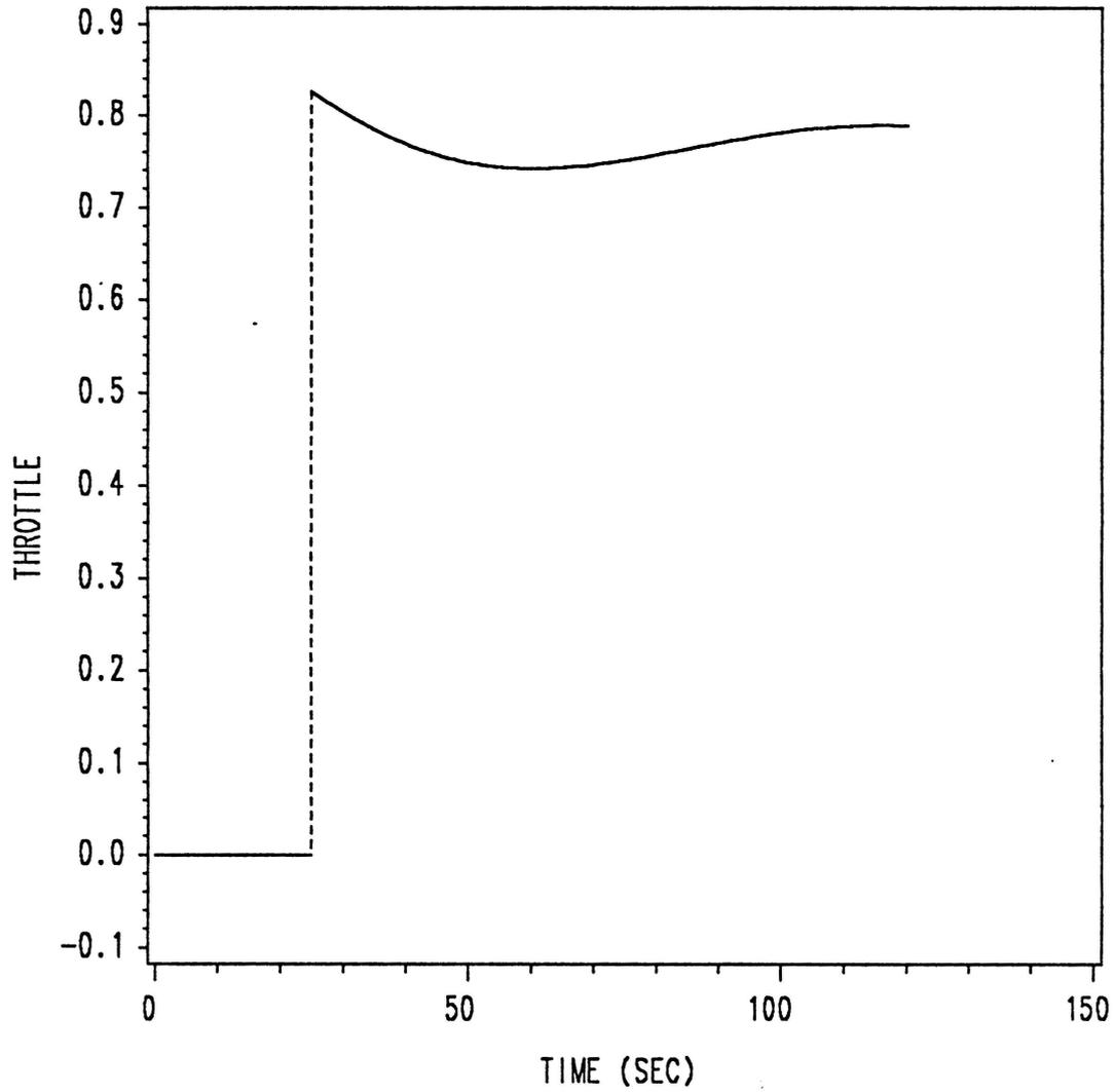
Figure 33. Throttle Time History for (Zero)Bang-Singular Control
