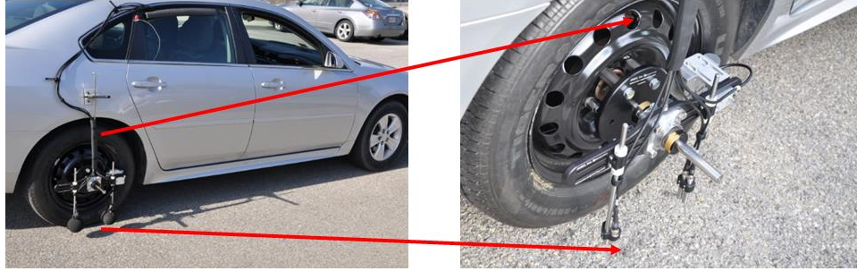
Figure 2- 4: OBSI system installed on the car.
