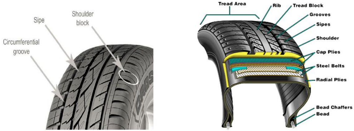
Figure A-2 Tire tread terminology. http://www.offroaders.com/tech/AT-MT-Tires/tire-tech.htm
