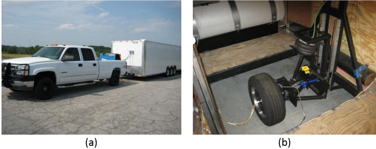
Figure 43: (a) test rig housing is attached to a tow vehicle that has a generator for power supply (b) test rig setup
