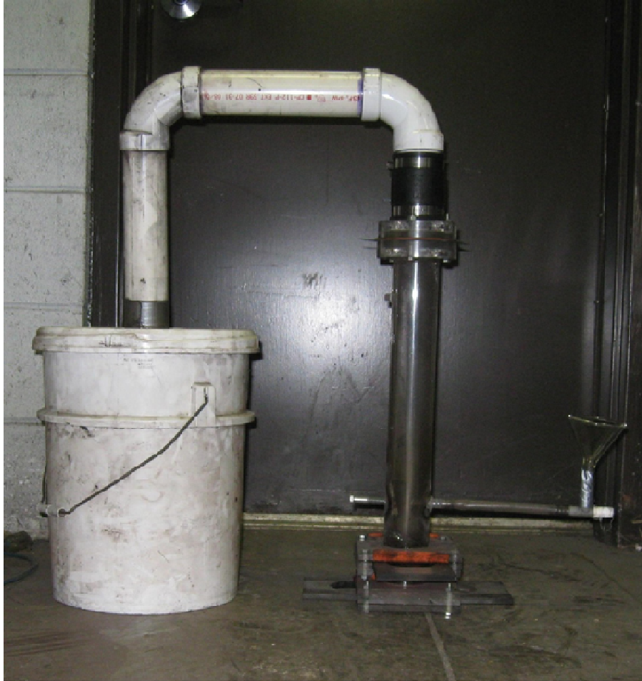
Figure 3-4. Static breaker device used for low temperature drying.
