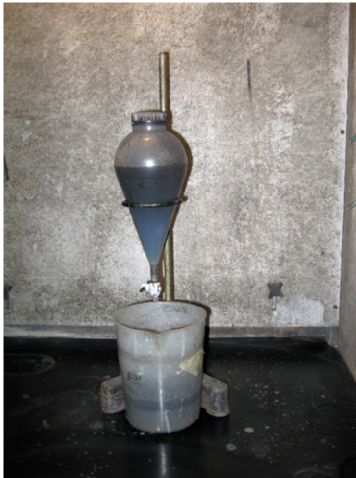
Figure 3-1. Separatory funnel used for laboratory testing.
