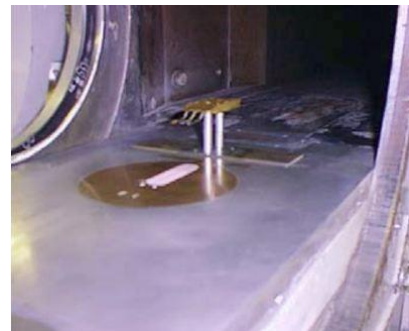
Figure 41: Triple-rake in Wind Tunnel
