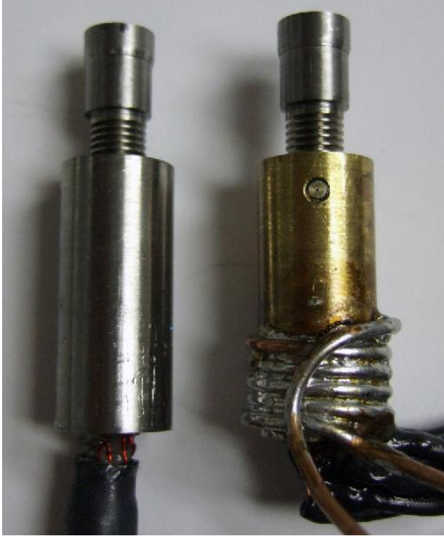
Figure 61: PT-2 , Build 2 (left), Build 3 with brass housing and soldered cooling tubes (right)
