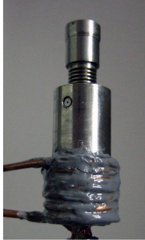
Figure 62: PT-2 , Build 4 with cooling tubes attached with metalized epoxy
