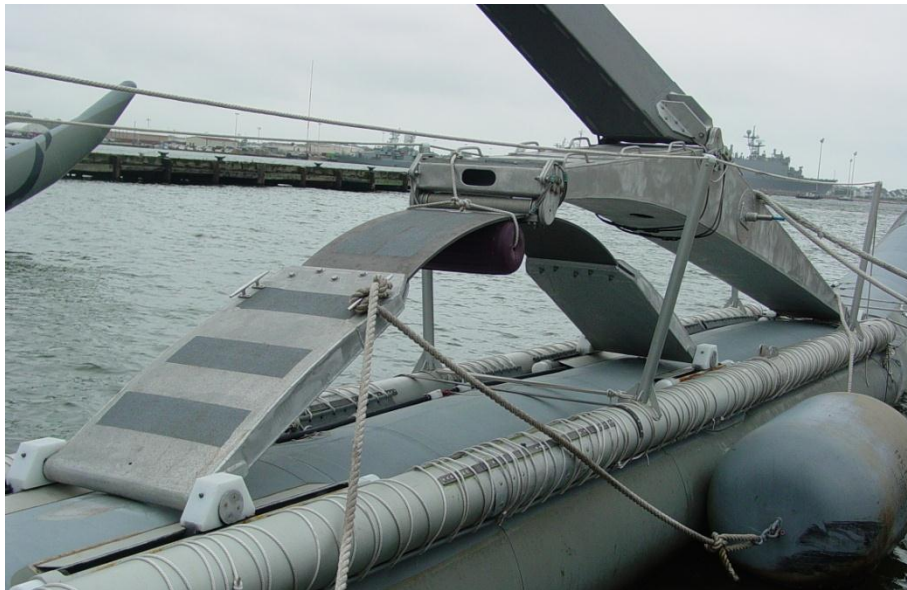
Figure 2.2. The springs positioned above each pontoon/arch attachment provide for mitigation of the heaving and pitching motions inherent to catamarans. Photo by author, 2011.
