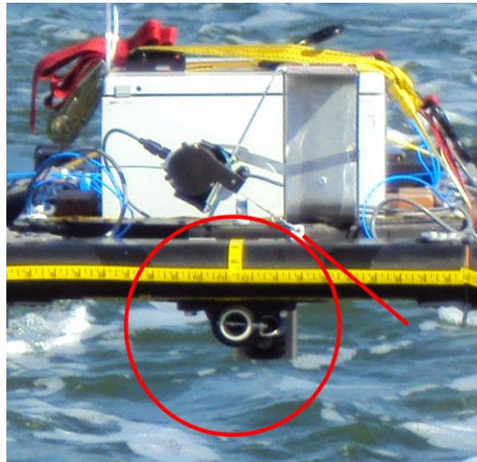
Figure 5.5. A string pot was installed using a custom mount to retain linearity of the measurement for both directions of motion. Photo by author, 2011.
