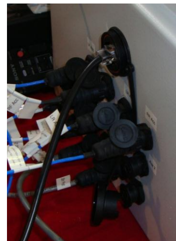
Figure 5.2. The battery and CompactRIO were situated within a water resistant box. Twelve waterproof connectors and an Ethernet port were also installed. Photo by author, 2011.
