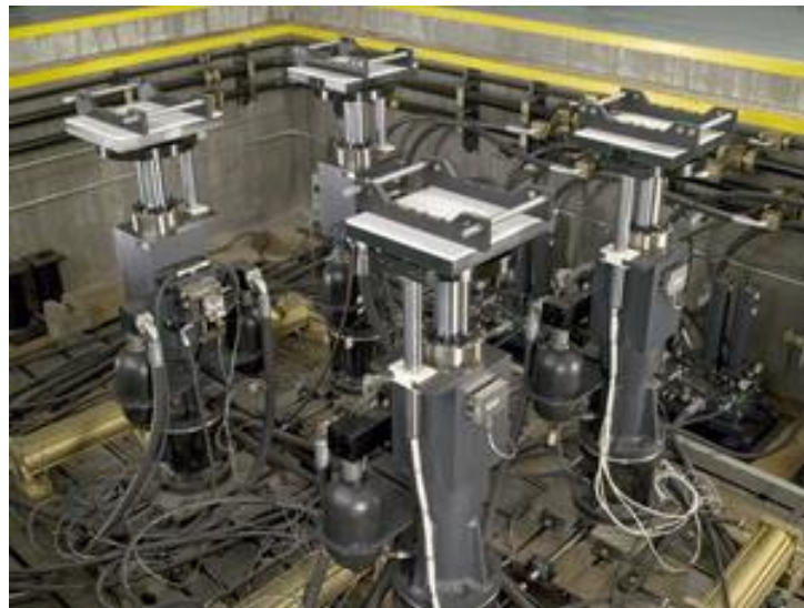
Figure 3.6. The under-workings of a shaker rig involve very large numerically controlled hydraulic pistons used to excite the vehicle's suspension. Photo by author, 2011.
