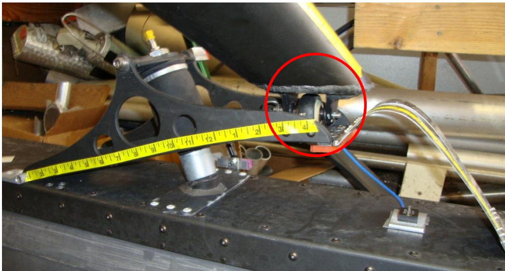
Figure 4.3. A spherical joint was utilized to attach the front arch and suspension and to allow for properly constrained motion of the pontoons relative to one another. Photo by author, 2011.
