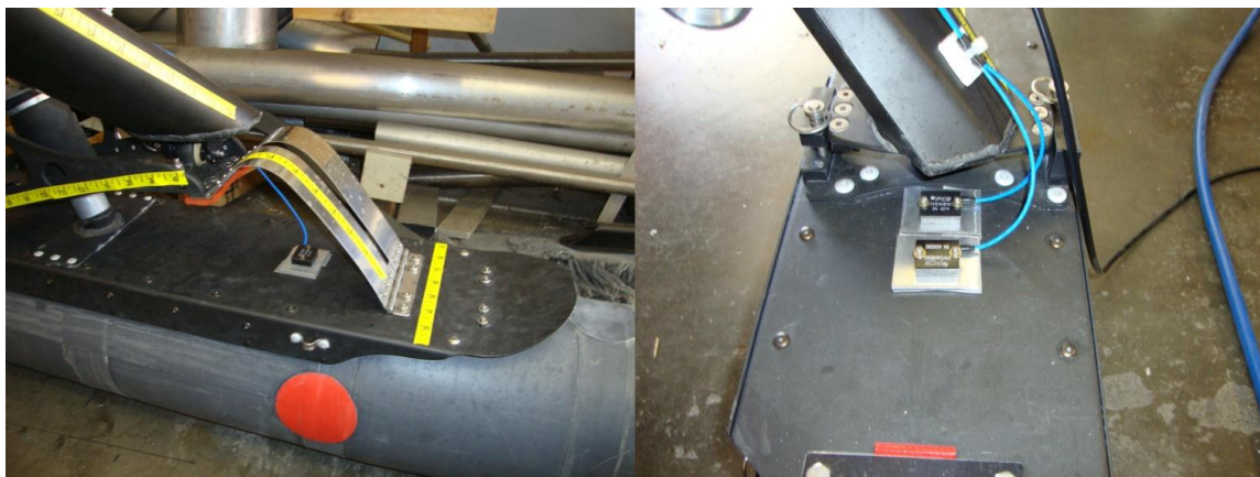
Figure 5.3. Accelerometers were mounted close to each arch attachment atop the rigid skis. Photo by author, 2011.
