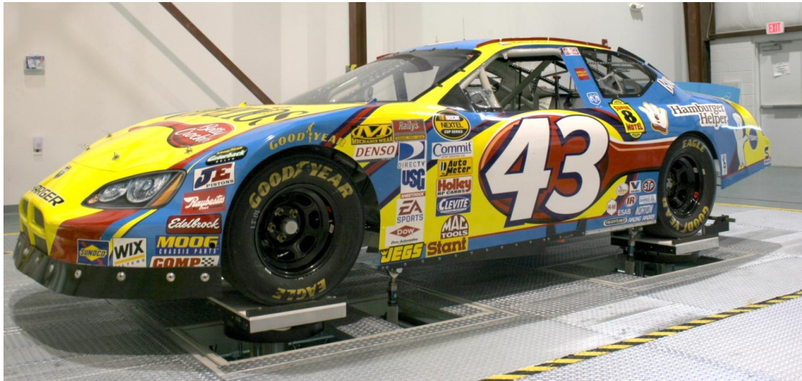
Figure 3.5. A stock car rests atop the input pads at the shaker rig located at VIPER in Danville, VA. Photo by author, 2011.
