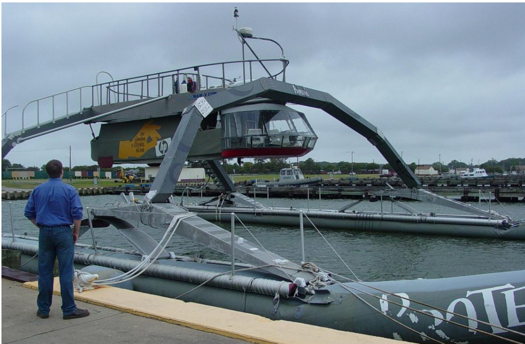
Figure 1.3. The Proteus is a WAM-V™ concept of catamaran which utilizes springs and a ball joint to help mitigate oceanic inputs to the cabin and improve passenger comfort. Photo by author, 2011.
