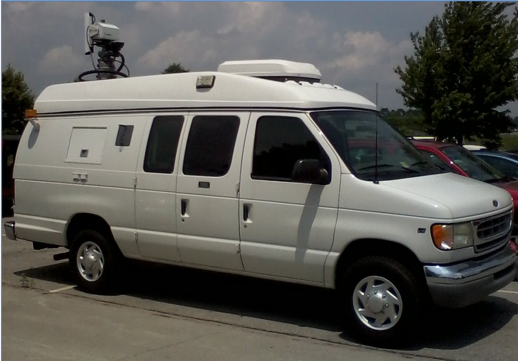
Figure 16: Research Vehicle with Camera in the Lowered Position
