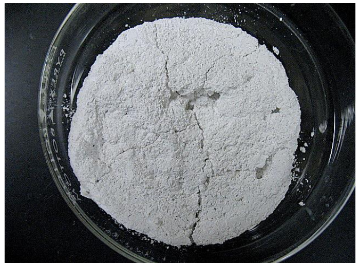
Figure 11 Dried green body subjected to cracking and volume shrinkage
