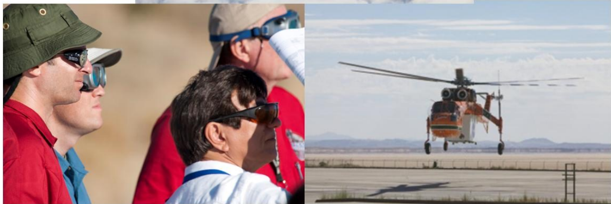
Figure 3.10: Erikson Airplane helicopter lifting off from NASA-Dryden and en-route to Edwards AFB test range carrying the ALHAT instrumentation pod. Members of the ground station at the hazard field are required to wear laser safety goggles due to the class IV non-eye-safe lasers being used.
