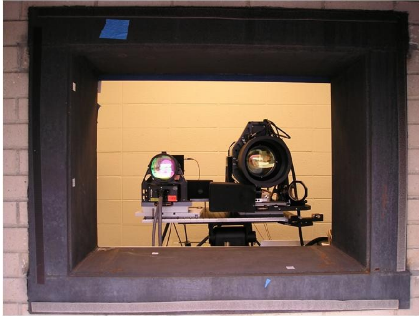
Figure 2.3: Fixed-FOV lidar (left) and var-FOV lidar (right) being characterized on the STR.
