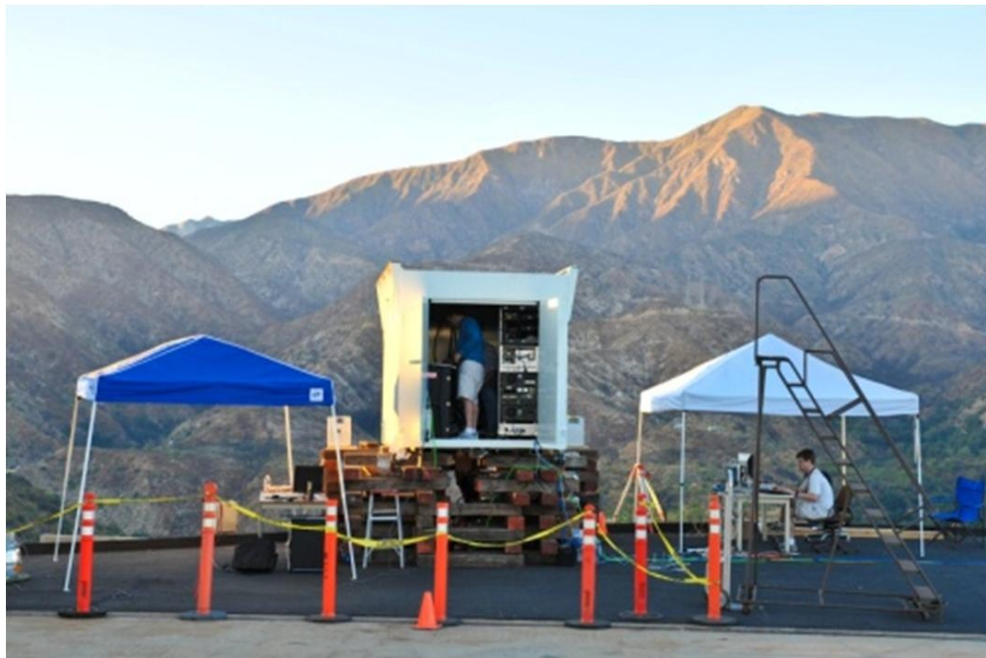
Figure 3.1: Both flash lidars along with support electronics are integrated into an instrumentation pod (center) with the other ALHAT GNC systems from NASA-JPL, NASA-JSC, and Draper Labs at the NASA-JPL mesa test range.
