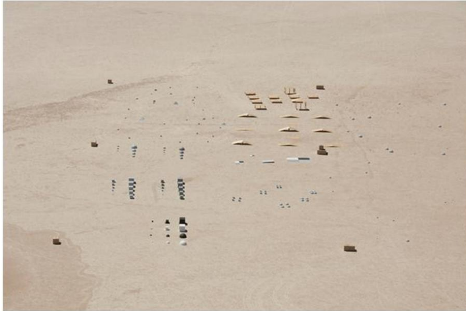
Figure 3.9: Aerial view of the complete hazard field situated on the Edwards AFB Rogers Dry Lake which consists of a host of square and hemispherical targets of varying size and spacing as well as safe-sites with no hazards designed to stress the lidar precision as well as the hazard detection algorithms. The hazard field is surrounded by the flat lakebed which serves as a target for the range precision runs.
