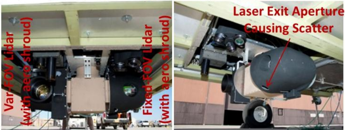
Figure 3.6: Instrumentation pod during preflight operations with rack systems being tested and with both flights lidars undergoing test. The flash lidars are deployed with the belly pod door open and each lidar covered by its own aerodynamic shroud. The fixed-FOV aerodynamic shroud, annotated on the picture, was the shroud whose laser exit opening was later found to be mis-aligned with the beam resulting in beam scattering and loss of laser exit energy along with the associated laser-scattering-induced pixel pre-triggering that required a reduction in lidar sensitivity.
