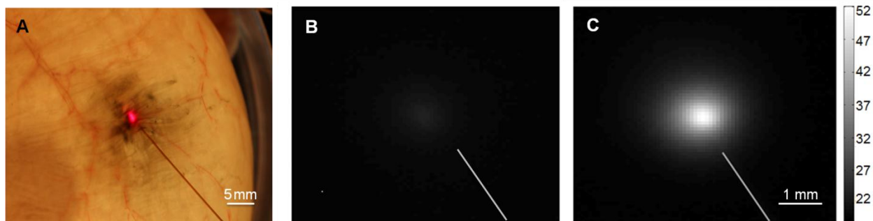
Figure 16: Irradiation from light-guiding, hollow-core microneedle after delivering SWNHs into the inflated bladder wall. (A) photograph showing microneedle position (Note: the red guide laser is visible), (B) thermograph of non-infused control, and (C) thermograph of SWNH perfused tissue. Color scale is in Celsius, white lines denote fiber path.
