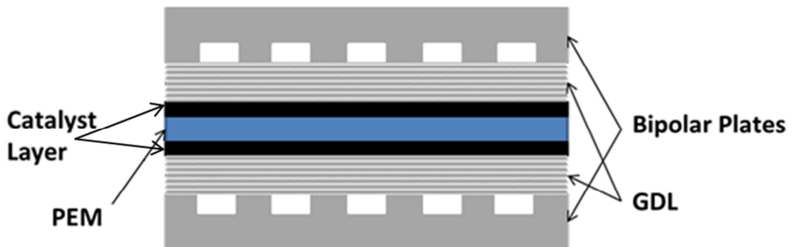
Figure 1-1: Basic schematic of a fuel cell. Not shown to scale.
