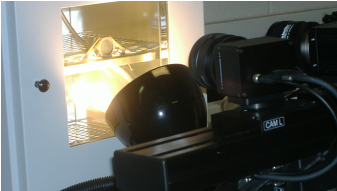
Figure 2-4: DIC blister fixture with front lighting for testing of PEMs
