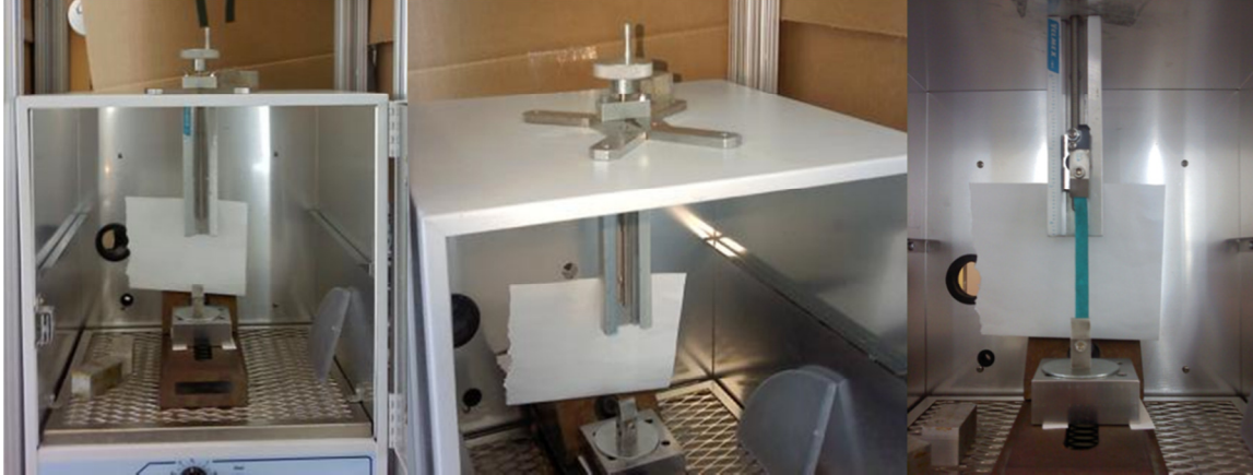
Figure D 1: Image of Poisson's ratio fixture. It is a simple screw driven relaxation fixture that can be manually set to a given displacement. The load is not measured in this fixture since there is no load cell
