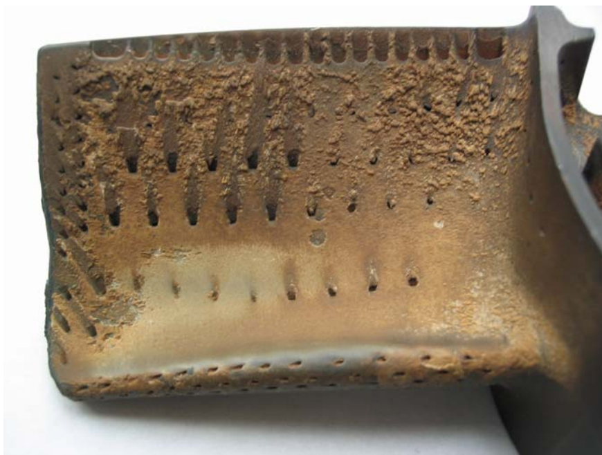
Figure 2.6. Sand has accumulated and blocked cooling holes on a V2500 turbine blade.
