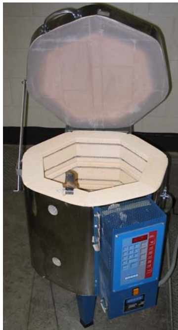
Figure 2.15. A ceramic kiln was used to simulate the metal and coolant temperatures reached in an actual turbine engine.
