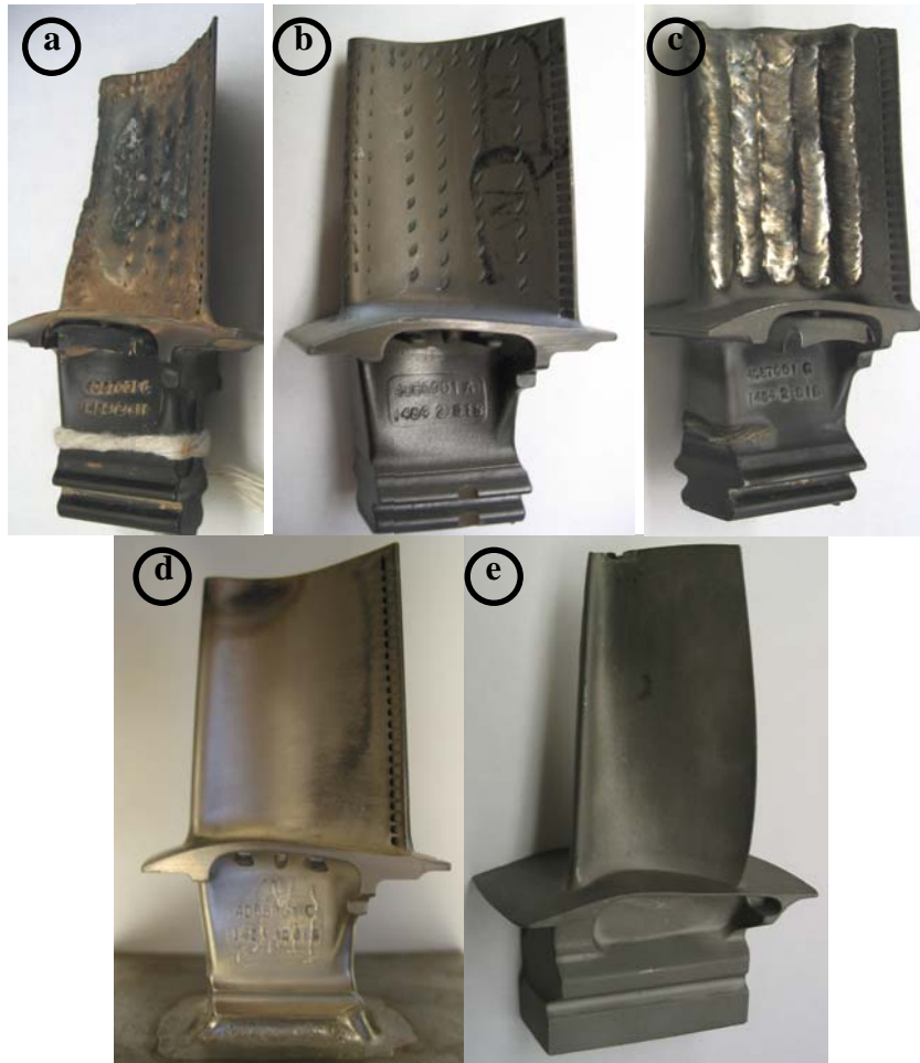
Figure 2.8. Turbine blades used in testing at Virginia Tech including, a) F-100-229-full field run blade, b) F-100-229-full new blade, c) F-100-229-TE field run blade, d) F-100-229-TE new blade, and e) F-119 microcircuit blade.
