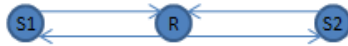
Figure 1.1: A two-way exchange channel. S_1 and S_2 are two source nodes which are out of reachable transmission range with each other. These two nodes exchange their information with the help of the relay node R .
