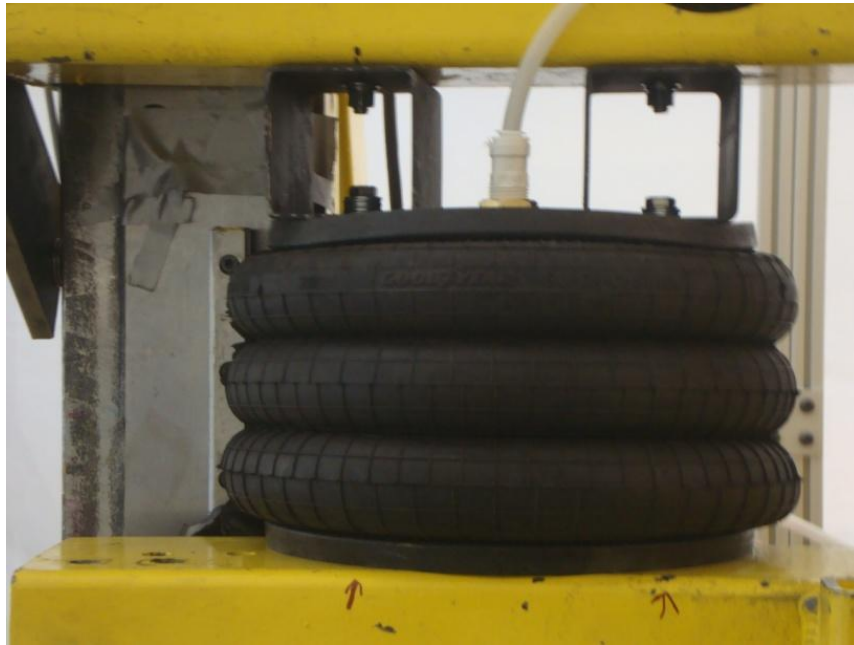
Figure 5-7. Close-up of the steel squares used to center the air springs on the crossbar above.
