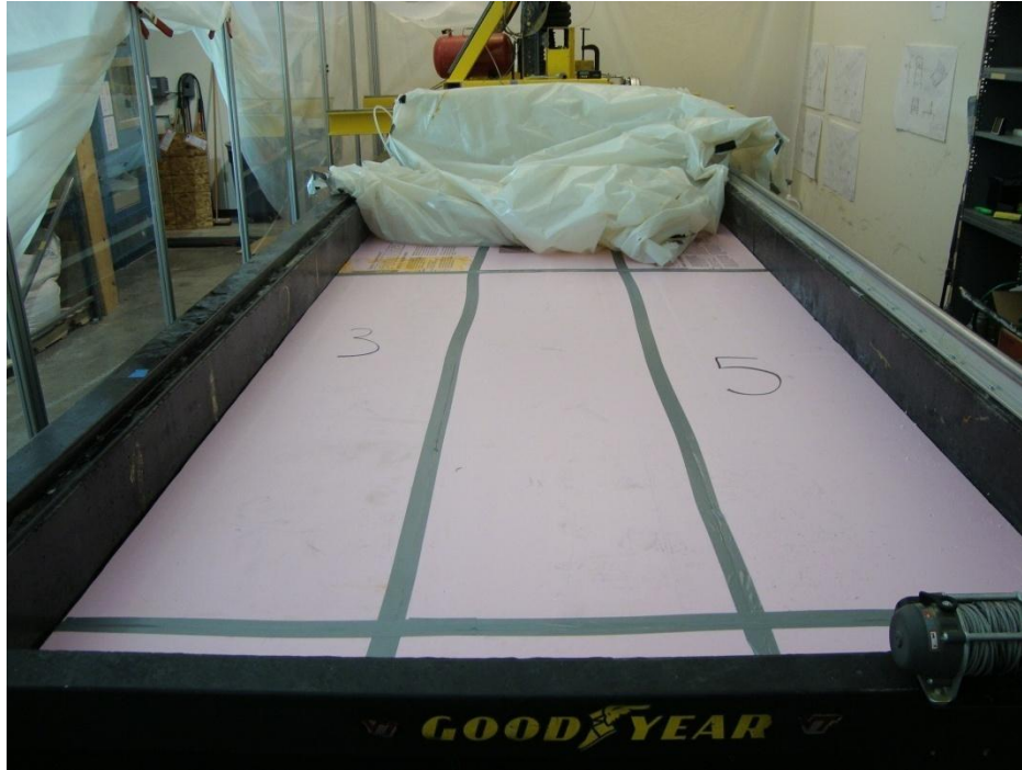
Figure 5-2. The foam insulation that sits above the steel C-channels.
