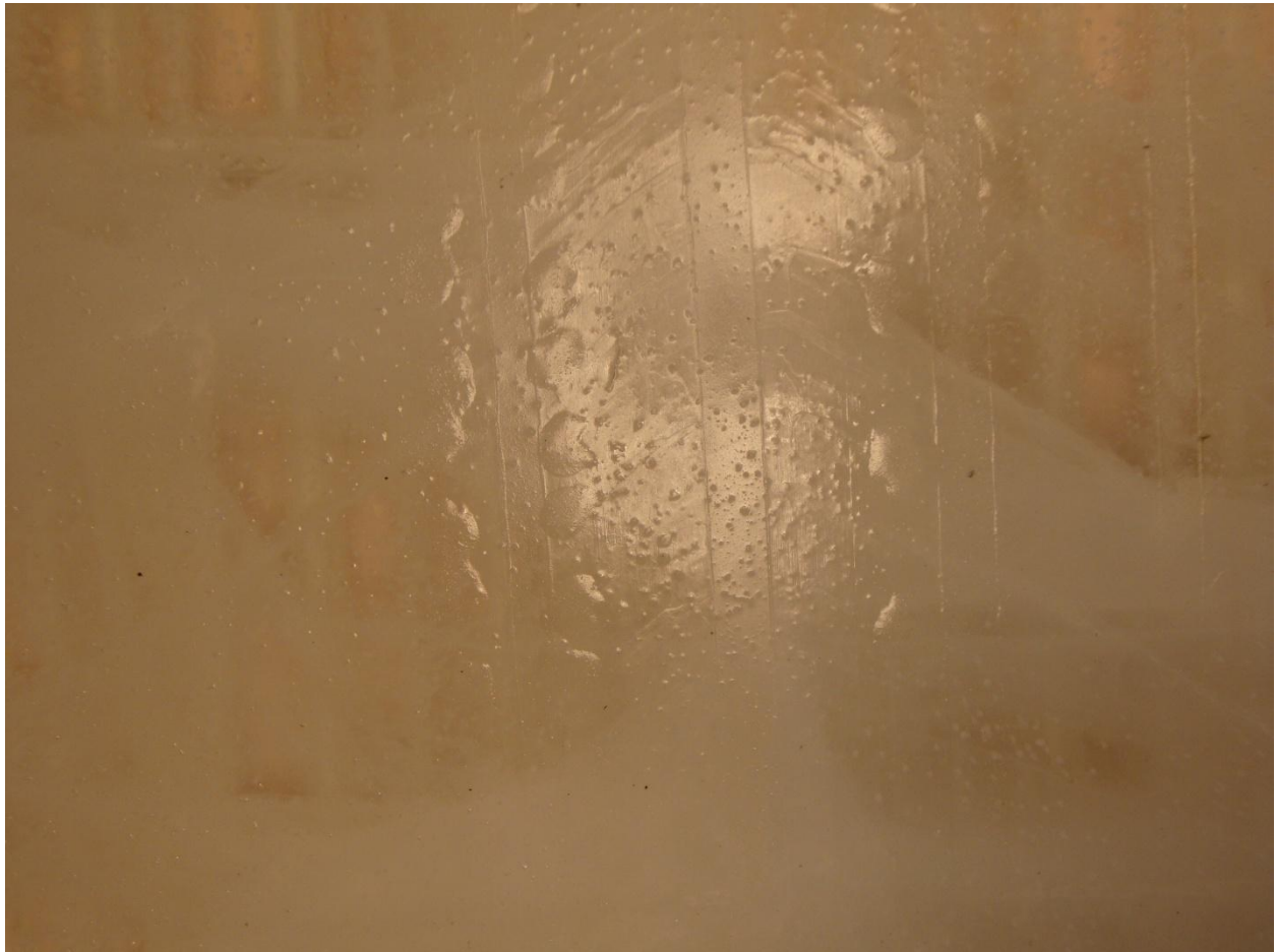
Figure 7-22. Image of the middle of the test surface with the generic winter tire tread pattern that left marks on the surface of the ice. Taken well after a run.
