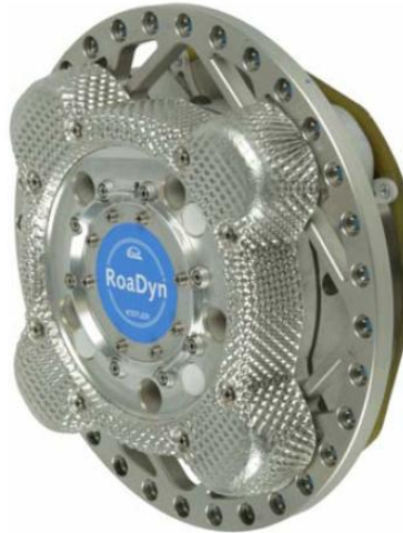
Figure 5-10. The dynamometer that contains the four load cell pairs [57].
