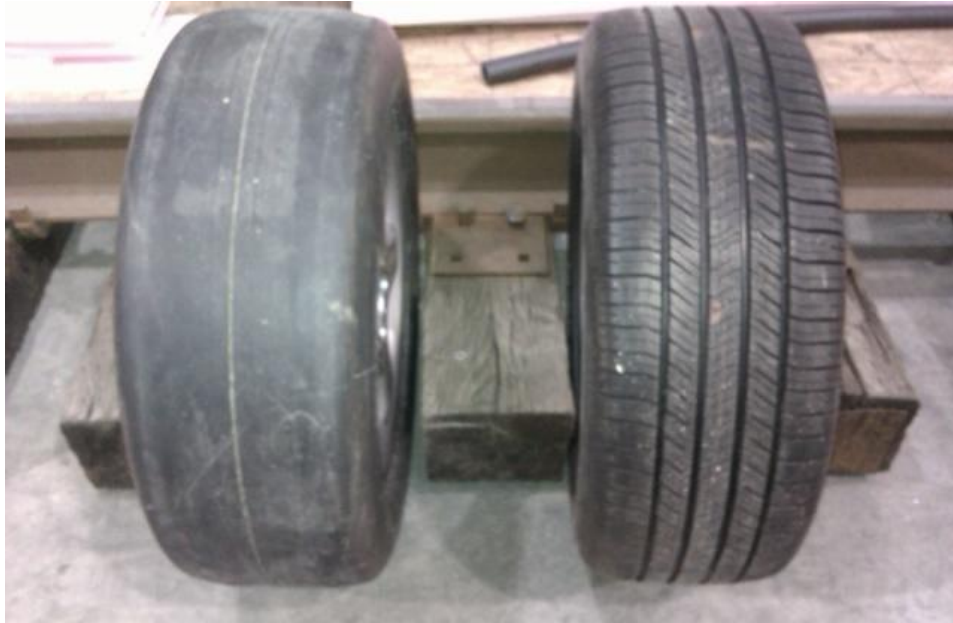
Figure 6-1. The two tires provided by Goodyear, with two different tread patterns: one bald tire and one tire with a generic winter tread pattern.
