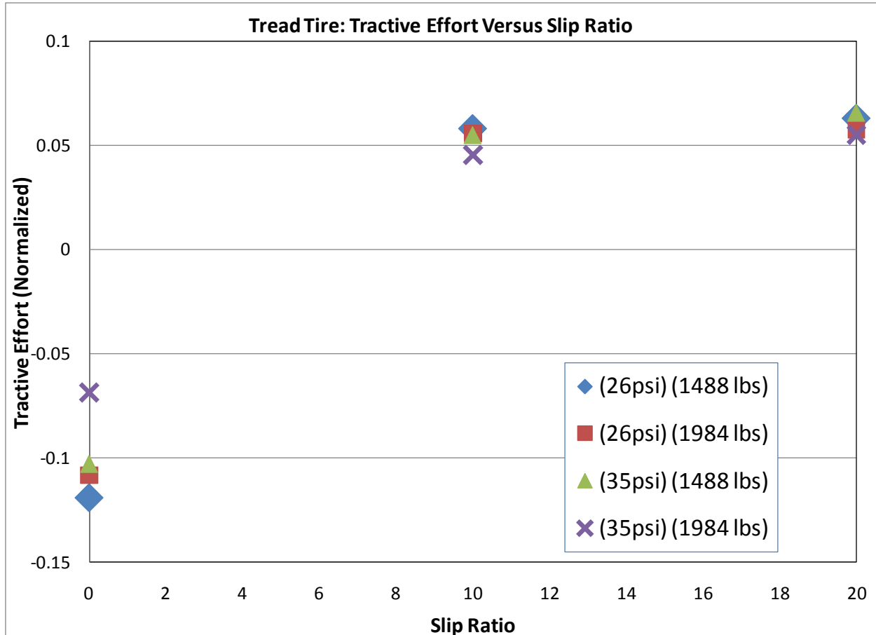
Figure 7-11. The normalized tractive force for the tire with tread.
