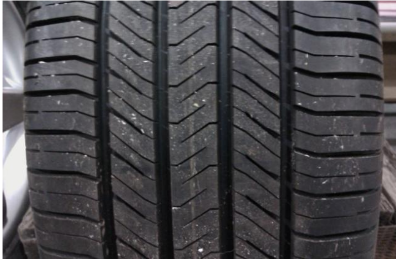
Figure 3-8. AVDL Goodyear pneumatic tire with generic winter tire tread pattern.
