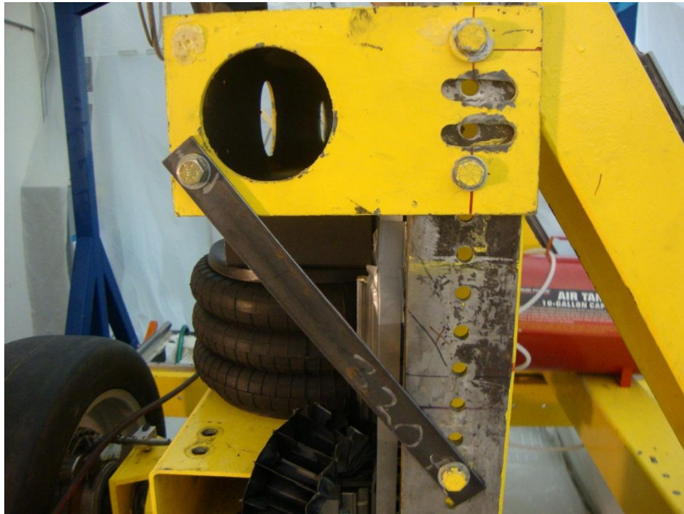
Figure 5-6. Side view of the reinforced crossbar.
