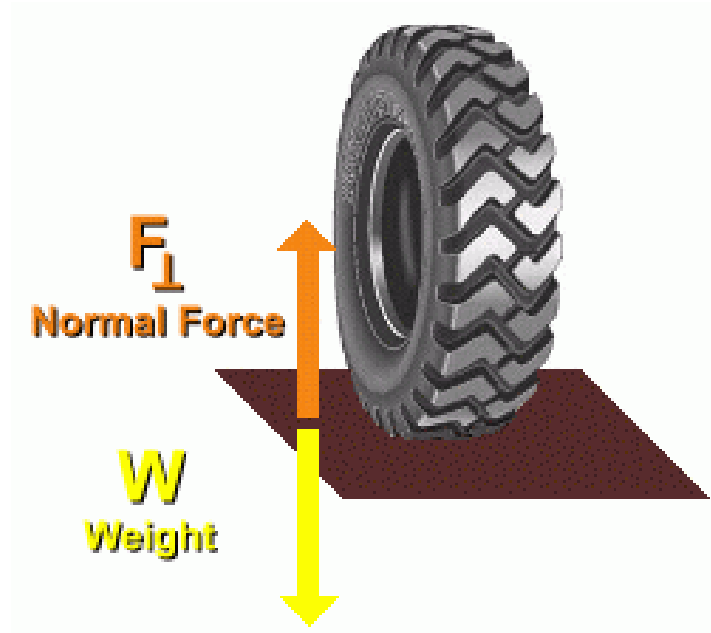
Figure 7-3. The normal force on the tire measured in the same direction as the positive z-axis by the Kistler hub [65].
