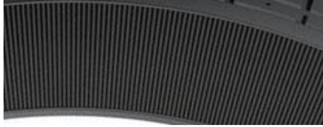
Figure 3-3. Vertical Serrated Band (VSB) sidewall design [27].
