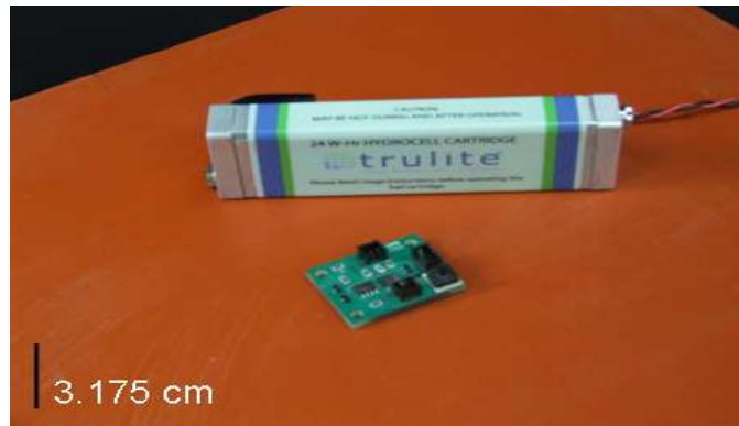
Figure 3.3. Trulite ® NaBH 4 tank fitting within the specified MAV fuselage parameters. The electrical chip in front of the tank is a flow controller.
