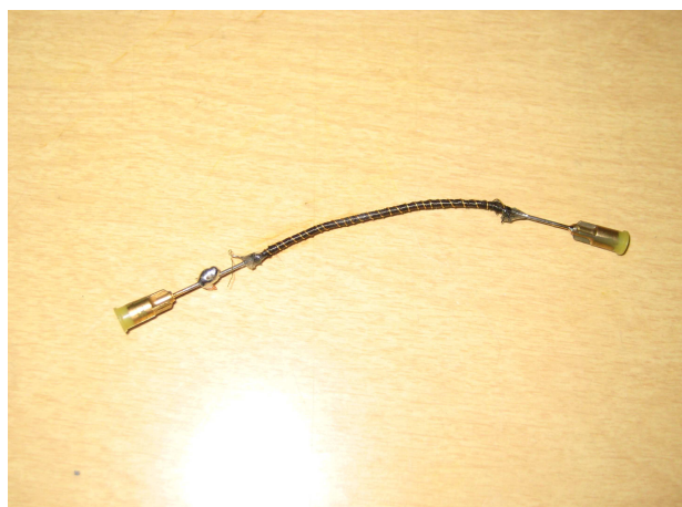
Figure 1.5. A tubular fuel cell ready for insertion into a stack.
