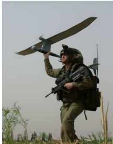
Figure 2.3. The Casper 200/250 backpack-able UAV designed by the Israeli defense forces (Defense Update, 2006; used with permission by N. Shental).
