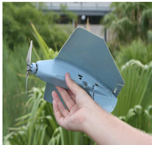
Figure 2.1. The Dragonfly MAV created by the University of Arizona (Paparazzi, 2006; fair use).
