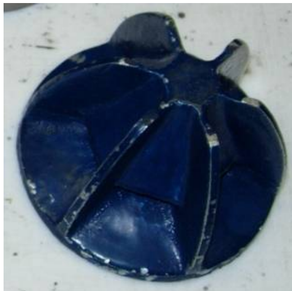
Figure 2.1: Typical rotor used in laboratory testing [Photo by Aaron Noble:10/24/2009].
