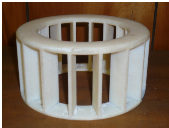
Figure 2.2: Generic stator used in laboratory testing [Photo by Aaron Noble:3/29/2010].
