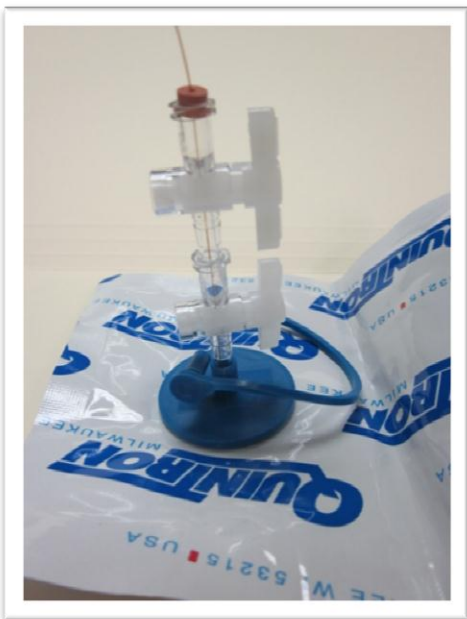
Figure 4 - \mu PC Capillary Tubing Inserted through Nested Valves, in Preparation for Sample Extraction from Bag
