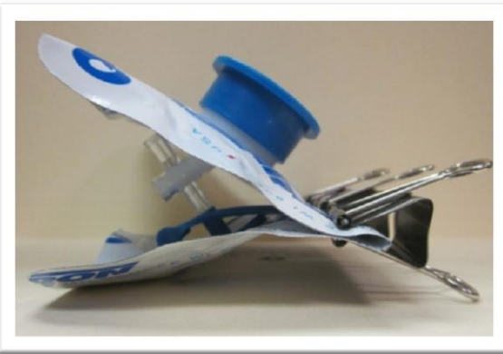
Figure 2 - Reduced Volume Sample Bag from Side with Valve
