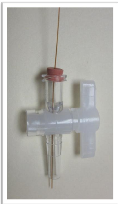
Figure 3 - \mu PC Capillary Tubing Inserted through Septum in Second Valve
