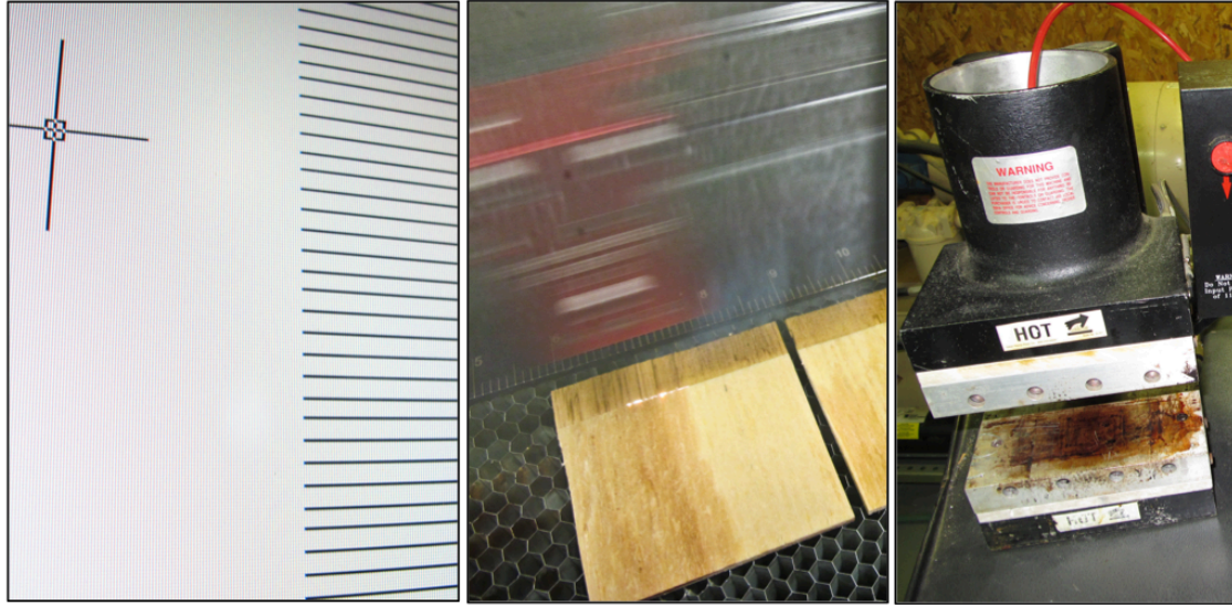
Figure 4.1: Illustration of method (a) screen shot of AutoCAD design (b) laser transferring design wood (c) mini hot press.
