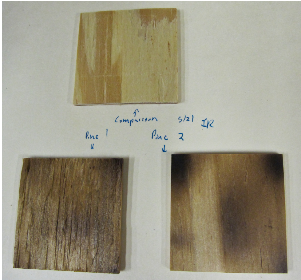
Figure A.3: Southern yellow pine samples (top) modified by IR lamp (bottom left) 2.5 min (bottom right) 5 min. Modification results in charring of the surface.
