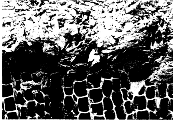
Figure 2.11: SEM comparison of band saw cutting (top of image) and laser irradiation (bottom of image) Used with the permission of Rightslink Copyright Clearance Center, Applied Surface Science Journal, 1998. [33].
