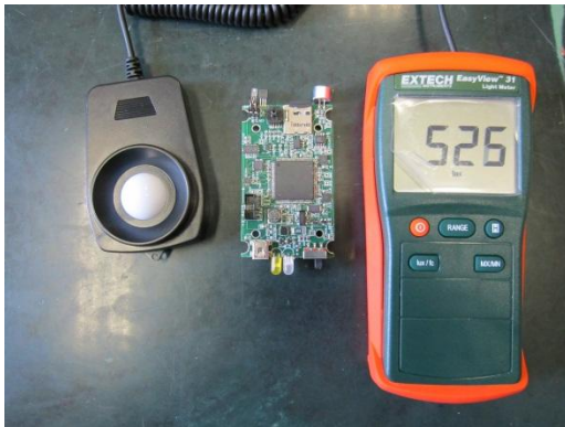
Figure 3-12. Light-meter calibration set-up
