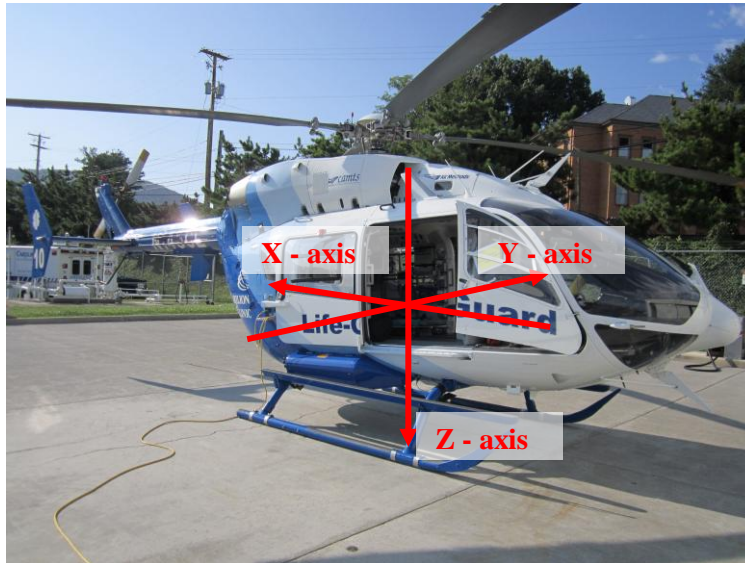
Figure 3-1. Orientation of the device's accelerometer with respect to the vehicle used for test flight
