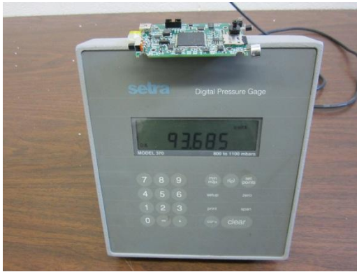
Figure 3-10. Barometer calibration set-up
