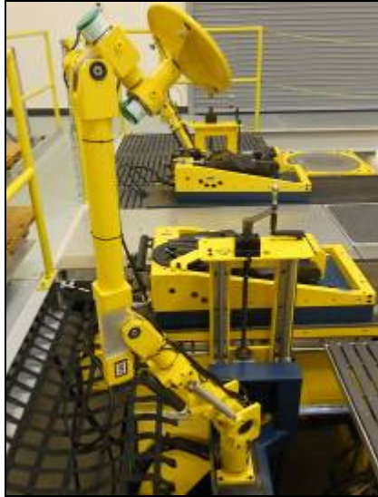
Figure 2.3: MTS K&C machine wheel motion sensor arm
