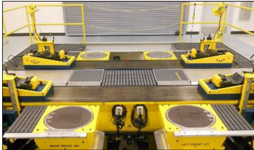
Figure 2.1: MTS K&C machine layout
