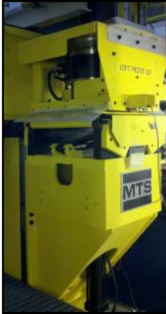
Figure 2.2: MTS K&C machine elevator platform
