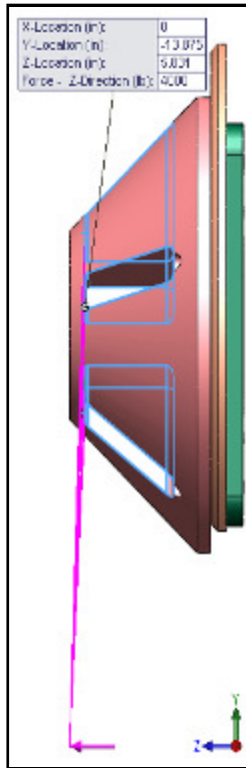
Figure F.10: Hub lateral loading
