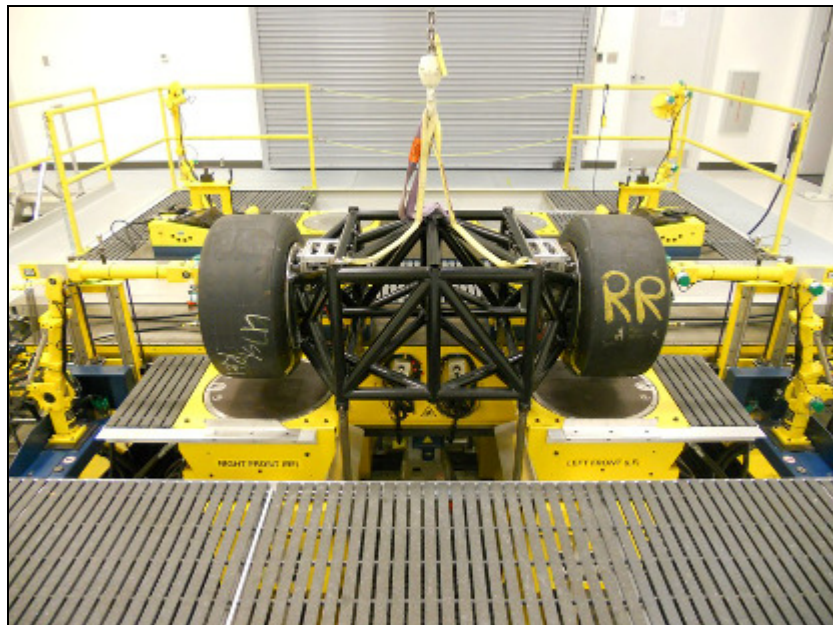
Figure 3.1: Fully constructed and installed test rig
