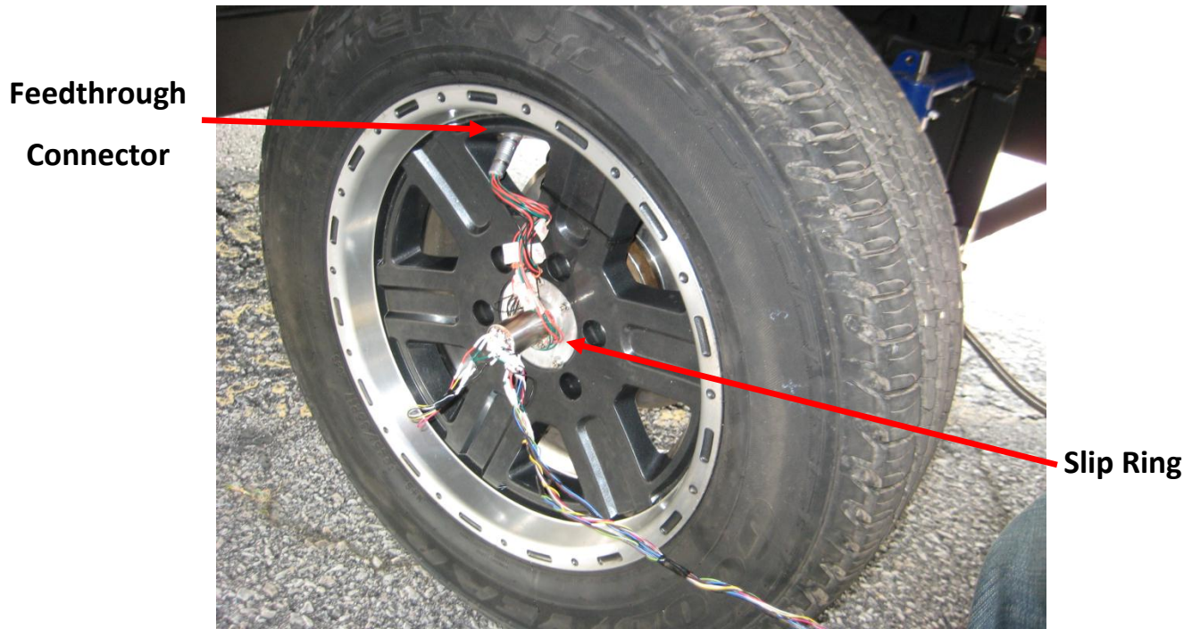
Figure 10. Photograph during testing of an intelligent tire showing the use of the slip ring.
