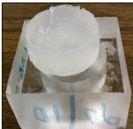
Figure 3.4: 90:10 (water:DMSO ratio) PVA hydrogel compression specimen.
