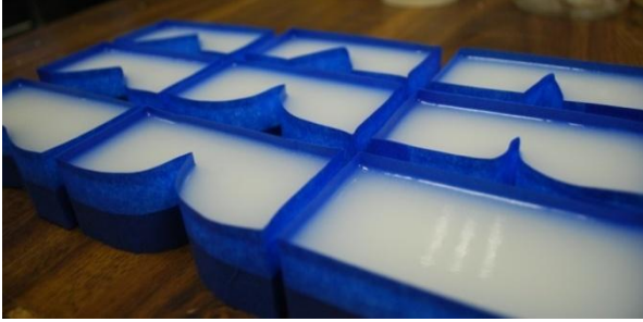
Figure 4.9: Test specimens after pouring super-soft silicone
