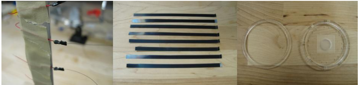
Figure 4.18: Parts for construction of internal structure. From left to right, SMA contractile wires, spring steel strips, and plastic rings.
