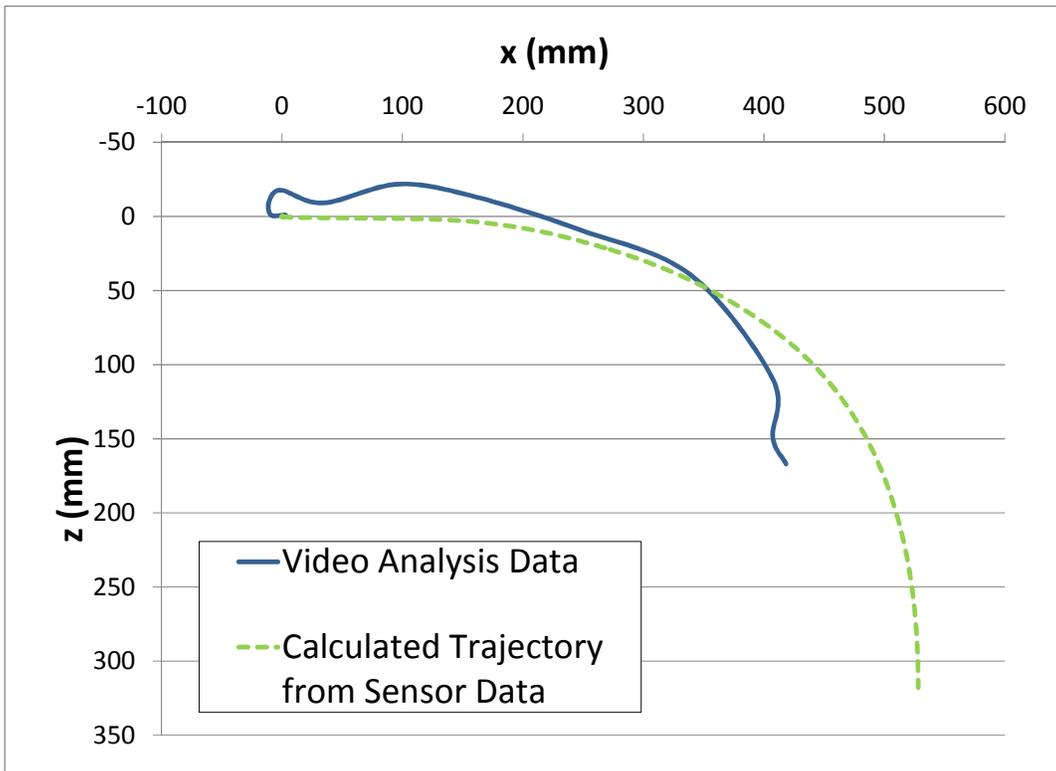
Figure 10. Head trajectories for UVA test 8380.
