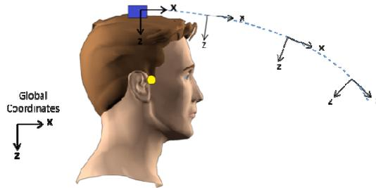
Figure 4. The orientation of the coordinate system changes as the head moves throughout a test.
