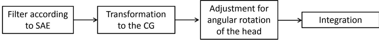
Figure 2. General procedure for obtaining head trajectory from acceleration and angular rate data.
