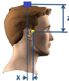
Figure 3. The distances between the sensor and the head CG defined by  $X$  and  $Z$ .
