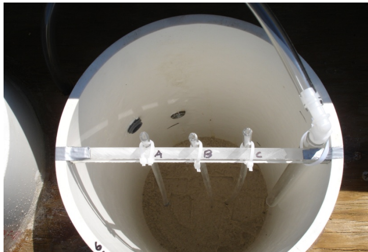
Figure 5. Sampling apparatus. A, B, and C refer to the location of the sampling depth within the column.
