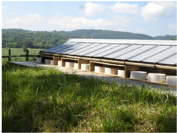
Figure 4. Column facility with custom-made plywood coverings.
