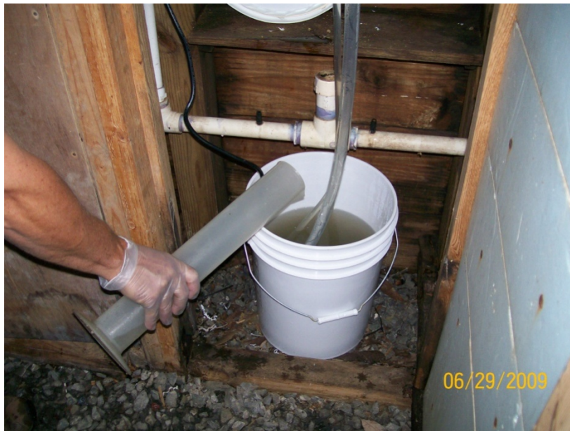
Figure 7. Adding wastewater influent to the reservoir buckets.
