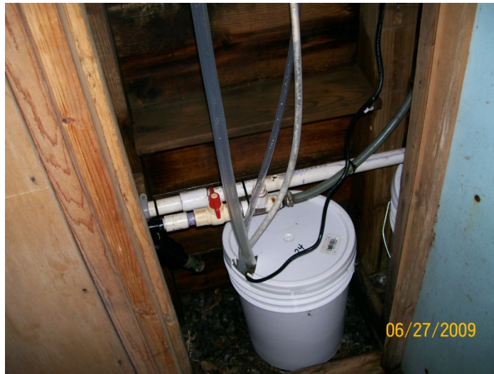
Figure 6. Picture of reservoir bucket. The large tubing is the overflow and the small clear tubing in the back is pumping the water back into the column.
